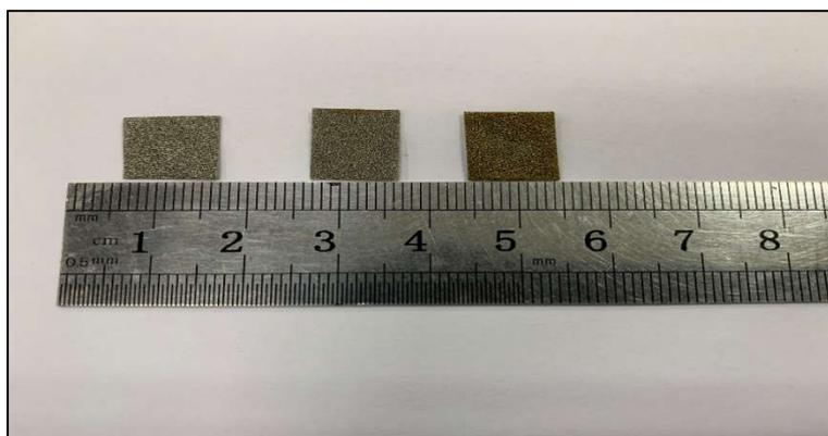
**Figure S4.** Digital pictures of Ni foam, I-NiFeOOH and E-NiFeOOH with  $1 \times 1 \text{ cm}^2$  area (from left to right).
