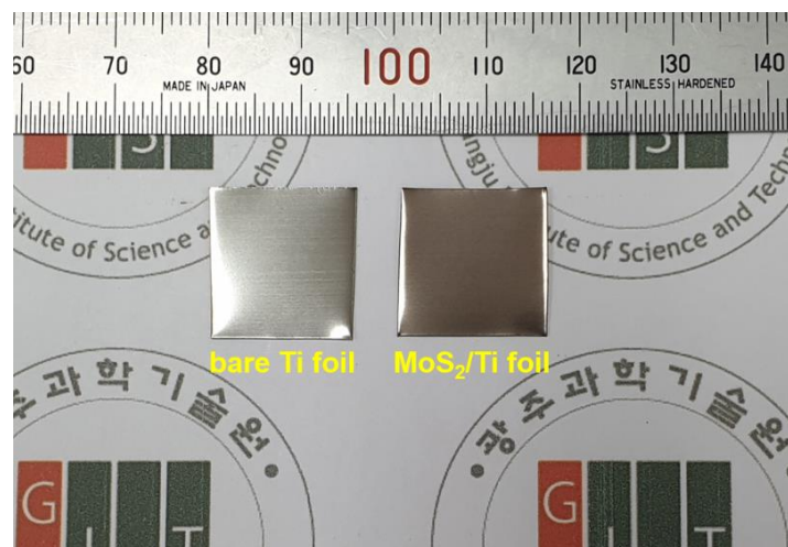
Fig. S2 Photograph of the bare Ti foil and MoS 2 /Ti foil.
