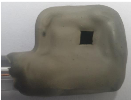
Fig. S14 Photographs of epoxy resin sealed MoS 2 /Ti foil/OHP photocathode. (a) Before and (b) after the measurement of PEC stability.
