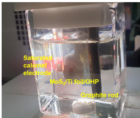
Fig. S6 Photograph of three-electrode configuration with MoS 2 /Ti foil/OHP, saturated calomel electrode (SCE), and graphite rod as working, reference, and counter electrode, respectively.
