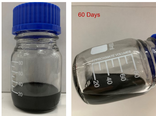
Fig. S5 Optical picture of the dispersibility of PDG nanosheets in water.
