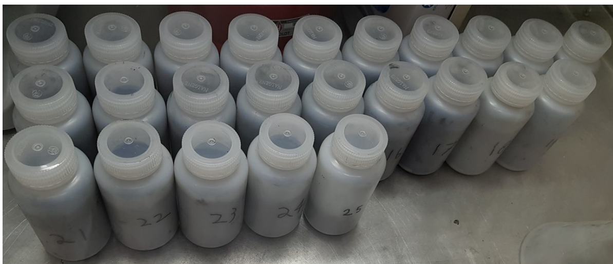
Figure S1. Annealed NCM811 powders acquired from 5 kg of USP precursors.
