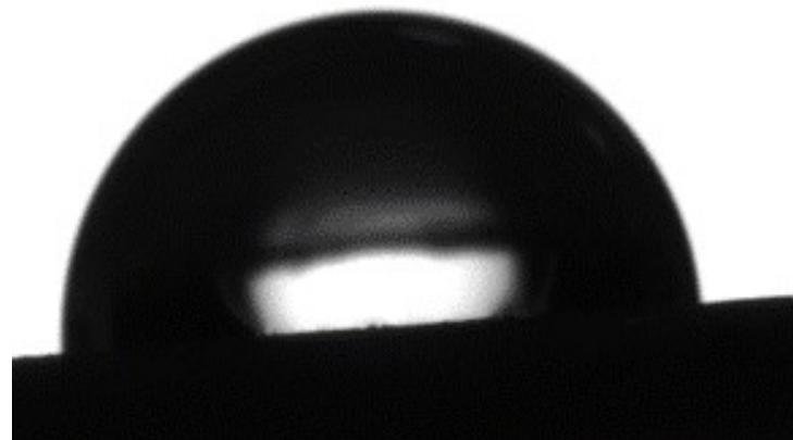
**Fig. S3:** Optical photograph of a water droplet (6 $\mu$ L) on pressed pellet of ZIF-9-I phase, showing contact angle around  $92 \pm 3^\circ$
