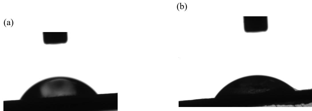
Fig. S8. Optical photograph of oil droplet on ZIF-9-III/PVDF membrane (a) vegetable oil, (b) Heptane.
