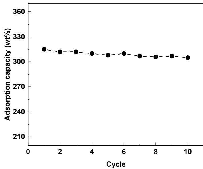
**Fig. S10:** Adsorption capacity of the ZIF-9-III@PVDF membrane over ten subsequent cycles and clearly shows significant adsorption capacity after 10 cycles of adsorption of vegetable oil.
