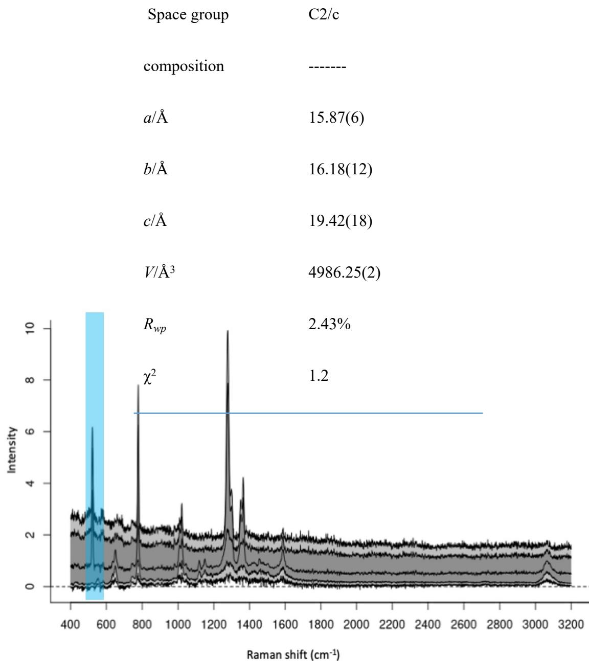
**Fig. S2:** Raman Spectrum of exfoliated ZIF-9-III
