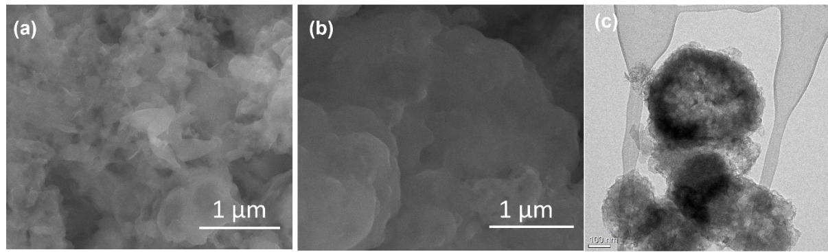
**Fig. S1:** (a-b) SEM (c) TEM images of bulk ZIF-9-III prepared through mechanochemical grinding
