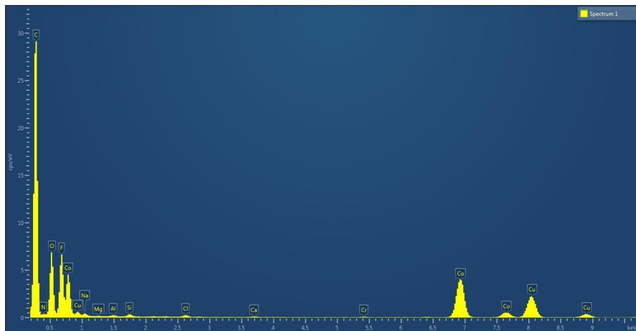
**Fig. S5:** EDS analysis of ZIF-9-III showing presence of Carbon, nitrogen, Cobalt, Oxygen and Fluorine elements of resultant membrane.
