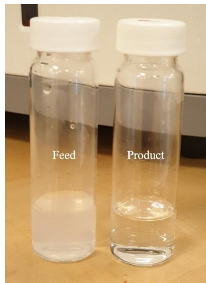
**Fig. S9:** Picture of oil/water emulsion (feed) and membrane purified oil (product).
