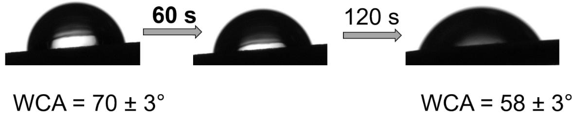
**Fig. S6:** Optical photograph of water droplet (6 $\mu$ L) on a PVDF membrane
