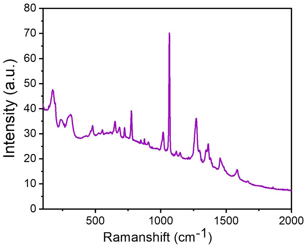
Fig. S11. Raman spectrum of ZIF-9@PVDF membrane showings Co-N bands at  $468\text{ cm}^{-1}$ , shows its structural integrity after oil-water separation.
