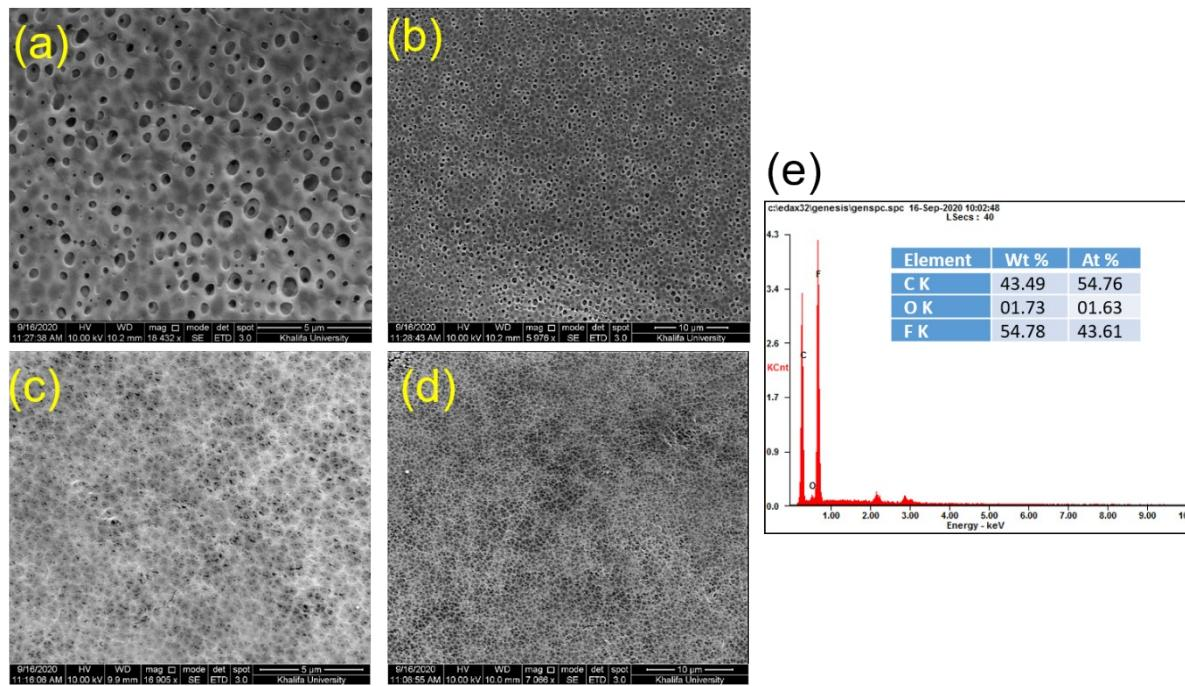
Fig. S4. SEM images of PVDF membrane (a-b) bottom view (c-d) top view; (e) EDS analysis
