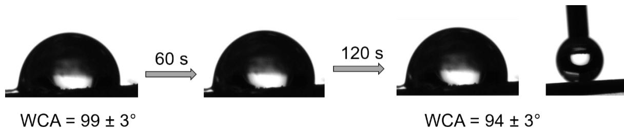
**Fig. S7:** Optical photograph of a water droplet (6 $\mu$ L) on a ZIF-9-@PVDF membrane
