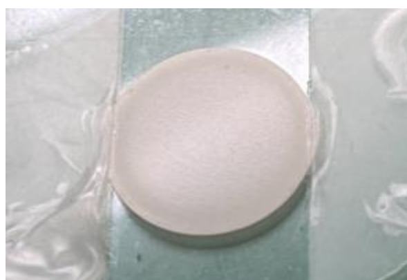
Figure S16. Left: spin-coating precursor solution. Right: AAO support coated with the APTS-GO/sPDMS layer. Both photos are for a 0.25 wt.% loading.
