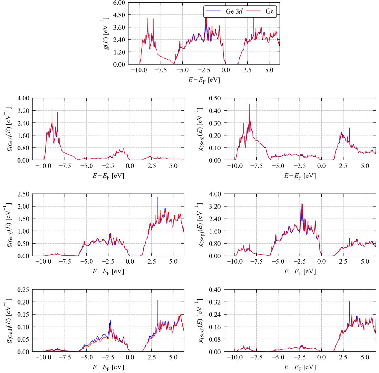
Figure S10: Calculated atom- and orbital-projected electronic density of states (pDoS) of GeSe obtained at the HSE 06 level of theory using pseudopotentials including the Ge  $3d$  electrons in the valence region (“Ge  $3d$ ”, blue) and treating them as core states (“Ge”, red).
