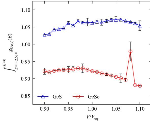
Figure S18: Numerical integral of the Ge  $s$  projected density of states (DoS) in Fig. S17 from  $E - E_F = -2.5 \rightarrow 0$  eV. The error bars show  $\pm$  the estimated error in the integrals. As noted above, the “spike” for GeSe at  $V = 1.09 V_{\text{eq}}$  is due to an artefact in the corresponding DoS function.
