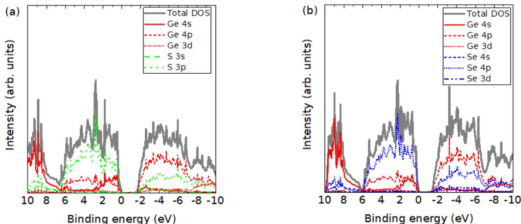
Figure S8: Atom- and orbital-projected electronic density of states (PDoS) of (a) GeS and (b) GeSe, without broadening or cross-section correction.
