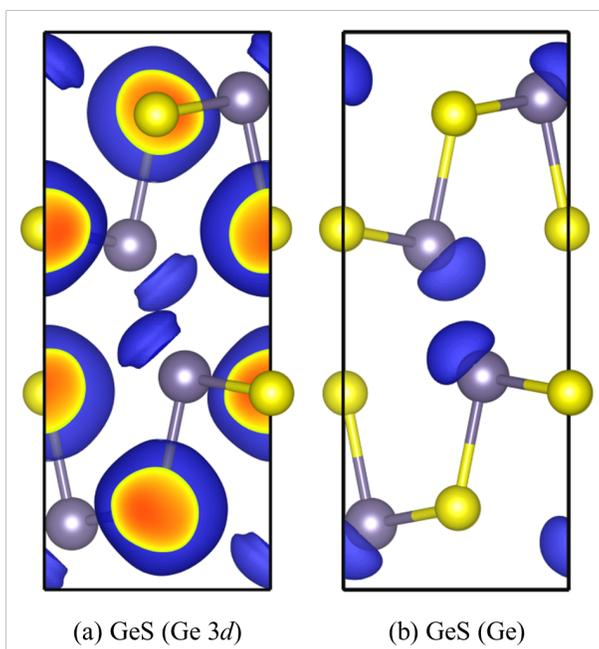
Figure S11: Electron localisation functions<sup>4</sup> of GeS calculated at the HSE 06 level of theory using pseudopotentials including the Ge 3*d* electrons in the valence region (a; “Ge 3*d*”) and treating them as core states (b; “Ge”). Isosurface levels: (a) 0.65, (b) 0.925. These images were prepared using VESTA.<sup>5</sup>
