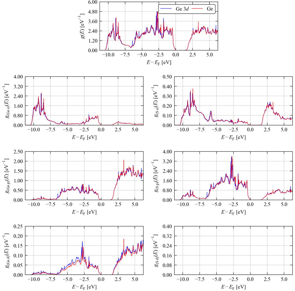
Figure S9: Calculated atom- and orbital-projected electronic density of states (pDoS) of GeS obtained at the HSE 06 level of theory from calculations using pseudopotentials including the Ge 3*d* electrons in the valence region (“Ge 3*d*”, blue) and treating them as core states (“Ge”, red).
