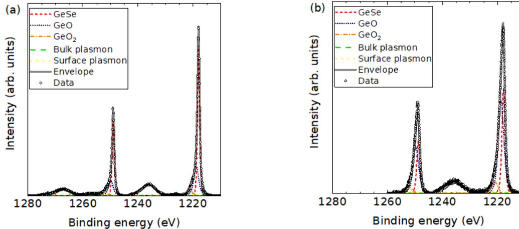
Figure S6: A comparison of (a) HAXPES and (b) XPS measurements and fits of the Ge  $2p$  region of the GeSe samples. The core level binding energies and FWHM are summarised in Table S3. The separations between peaks are supported by *in situ* XPS measurements (Figure S7), which showed larger amounts of contamination. Both sets of spectra have had a Shirley background subtracted.
