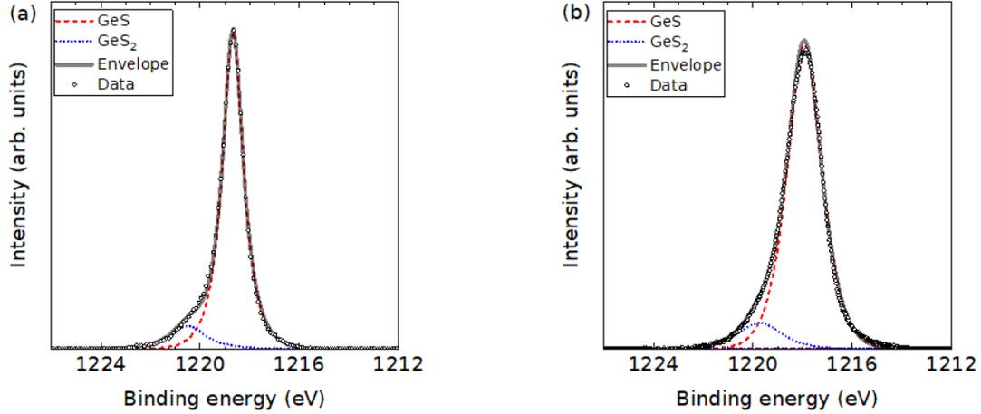
Figure S4: A comparison of (a) HAXPES and (b) XPS measurements and fits of the Ge  $2p$  region of the GeS samples. The core level binding energies and FWHM are summarised in Table 1. The separations between peaks are supported by *in situ* XPS measurements (Figure 5), which showed larger amounts of contamination. Both sets of core level spectra have had a Shirley background subtracted.
