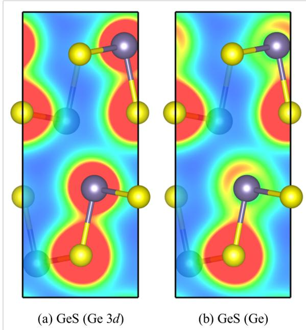
Figure S13: Charge density of GeS calculated at the HSE 06 level of theory using pseudopotentials including the Ge 3d electrons in the valence region (a; “Ge 3d”) and treating them as core states (b; “Ge”). Each image shows a cut through the  $ab$  plane at a distance of  $0.75c$  from the origin, which bisects two of the Ge atoms. The cut shows contour values in the range of  $[0, 0.5] e \text{ \AA}^{-3}$ . These images were prepared using VESTA.<sup>5</sup>
