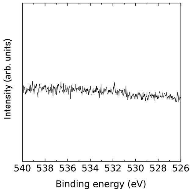
Figure S3: Core-level spectrum of the GeS sample in the O 1s region. A peak near 531 eV is expected if oxygen is present in the sample. This spectrum therefore indicates minimal oxygen contamination at the surface of the sample and accounts for the absence of Ge oxide features in the GeS core level spectra shown in the main manuscript and below.
