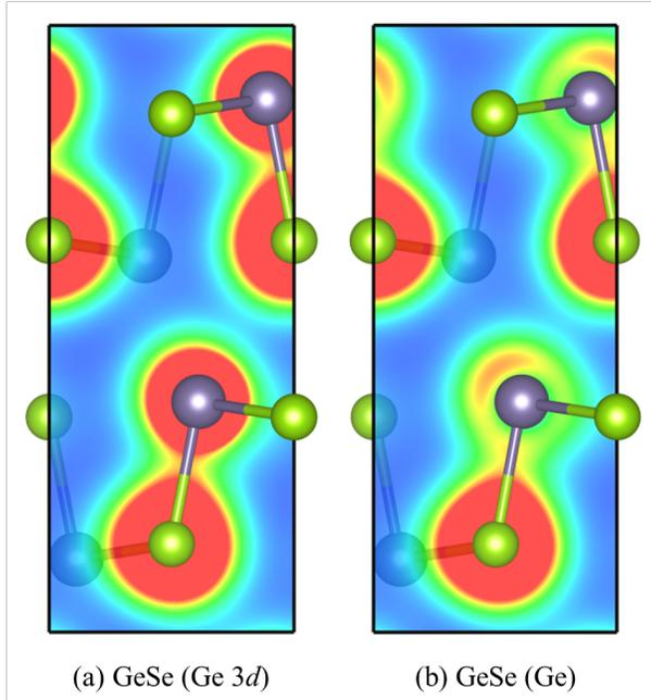
Figure S14: Charge density of GeSe calculated at the HSE 06 level of theory using pseudopotentials including the Ge 3d states in the valence region (a; “Ge 3d”) and treating them as core states (b; “Ge”). Each image shows a cut through the  $ab$  plane at a distance of  $0.75c$  from the origin, which bisects two of the Ge atoms. The cut shows contour values in the range of  $[0, 0.5] e \text{ \AA}^{-3}$ . These images were prepared using VESTA.<sup>5</sup>
