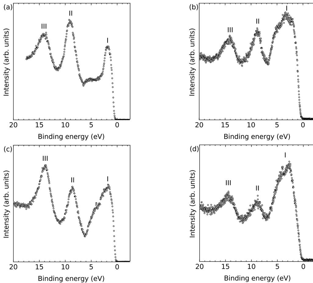
Figure S1: (a) and (b) show HAXPES and XPS measurements of GeS, respectively, while (c) and (d) show HAXPES and XPS measurements of GeSe. Peaks I, II and III are labelled to correspond to how they are referred to in early reports on the valence bands of GeS and GeSe. Peak I was initially thought to be composed of S  $3p$ /Se  $4p$  and Ge  $4p$  orbitals, Peak II of Ge  $4s$  orbitals, and Peak III of S  $3s$ /Se  $4s$  states.
