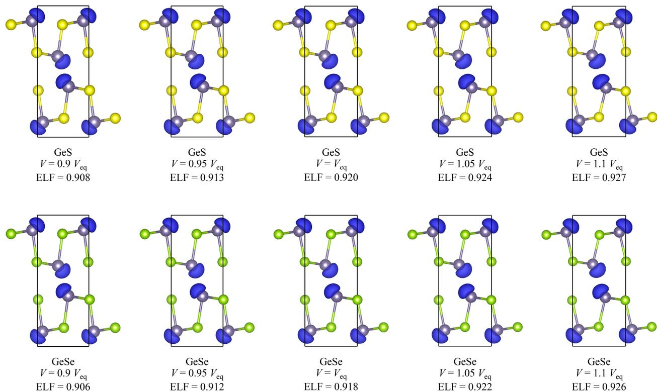
Figure S19: Calculated electron-localisation functions (ELFs) of GeS and GeSe at volumes between  $\pm 10\%$  of the equilibrium volume  $V_{\text{eq}}$ . The ELF isosurface values have been adjusted to show the Ge lone pairs at similar spatial extents. These calculations were performed at the HSE06 level of theory and using pseudopotentials treating the Ge  $3d$  electrons as core states. The images were prepared using VESTA.<sup>5</sup>
