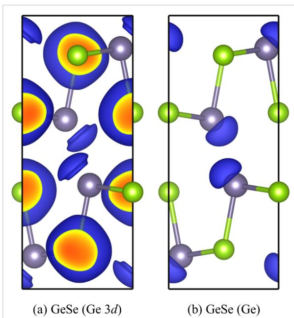
Figure S12: Electron localisation functions<sup>4</sup> of GeSe calculated at the HSE 06 level of theory using pseudopotentials including the Ge 3*d* electrons in the valence region (a; “Ge 3*d*”) and treating them as core states (b; “Ge”). Isosurface levels: (a) 0.65, (b) 0.925. These images were prepared using VESTA.<sup>5</sup>
