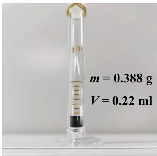
Fig. S16 The photograph on tap density measurement of NCO@NC-FMS.
