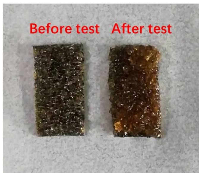
Figure S7. The typical optical photographs before and after HER test for PVP@Pt/Ni(OH) 2 @NF
