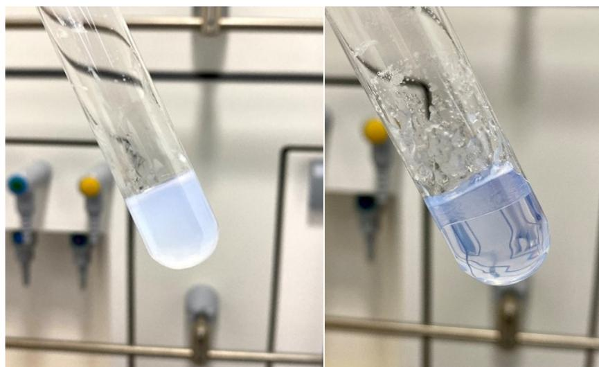
Figure S2: PP-solvogel with relatively high polymer content (35%)
