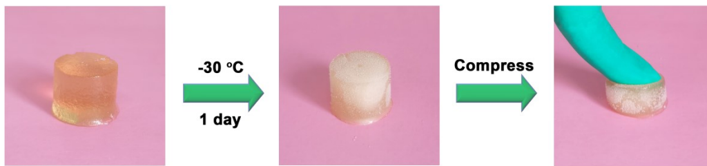
Figure S6. Photographs of the hydrogel (0:20) after storage at -30 °C for 1 day.
