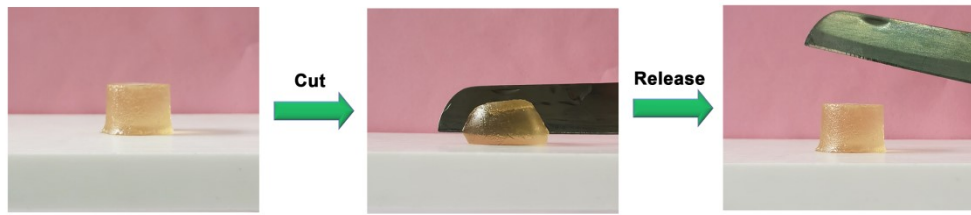
Figure S1. The PAM/CS-PA hydrogels (0:20) resisted the cut with a blade.
