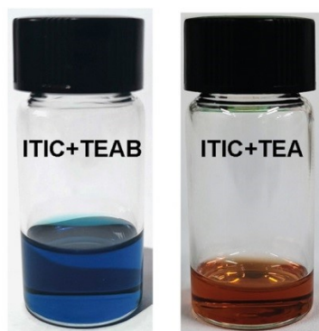
Fig. S9 The ITIC solution mixed with tetraethylammonium bromide (TEAB) and triethylamine (TEA) for 10 days under room temperature.
