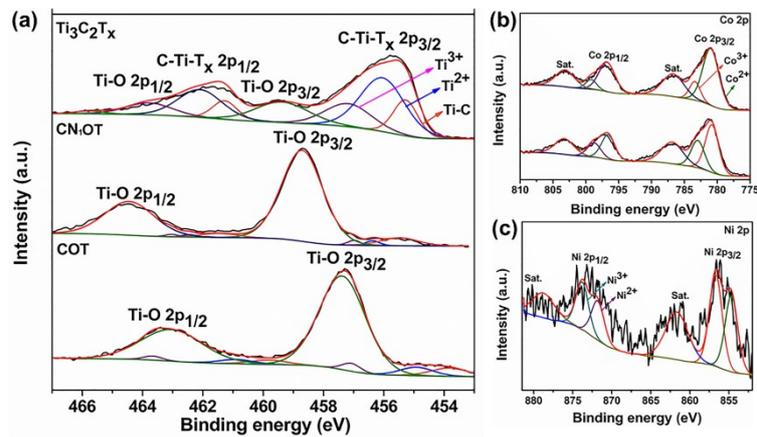
**Fig. S4** High-resolution XPS spectra of (a) Ti 2p, (b) Co 2p and (c) Ni 2p of Ti<sub>3</sub>C<sub>2</sub>T<sub>x</sub>, COT and CN<sub>1</sub>OT.
