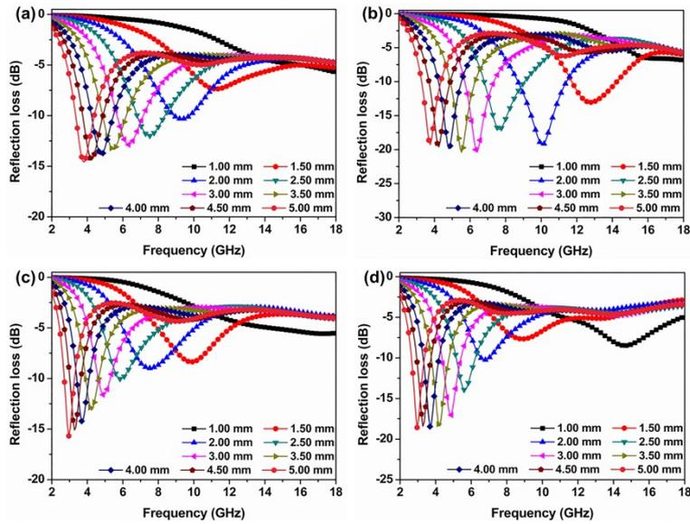
Fig. S11 2D RL curves of pure MXene with different filler content in PVDF, (a) 5 wt%, (b) 10wt%, (c) 15wt% and (d) 20wt%.
