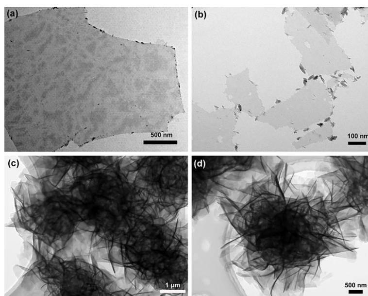
**Fig. S1** TEM image of (a,b) Ti<sub>3</sub>C<sub>2</sub>T<sub>x</sub> nanosheets and (c,d) CM flowers.
