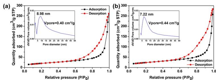
**Fig. S5**  $N_2$  adsorption-desorption isotherm and pore size distribution of (a) CO and (b)  $CN_1O$  composites, respectively.
