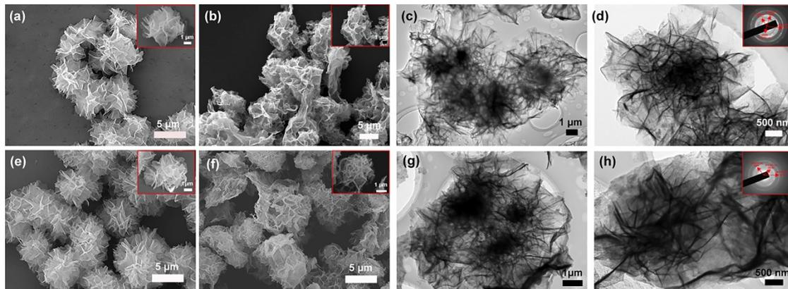
**Fig. S3** SEM images of (a) CN<sub>5</sub>M, (b) CN<sub>5</sub>OT, (e) CN<sub>9</sub>M and (f) CN<sub>9</sub>OT composites, TEM images of (c,d) CN<sub>5</sub>OT and (g,h) CN<sub>9</sub>OT.
