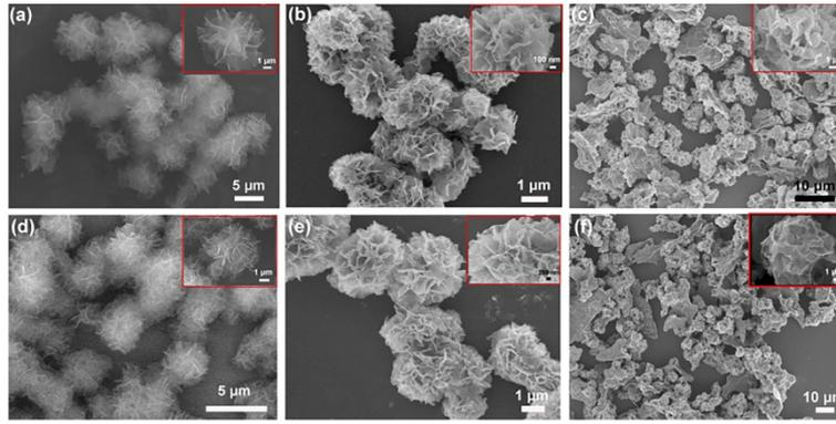
**Fig. S2** SEM image of various samples, (a) CM, (b) CO, (c) COT, (d) CN<sub>1</sub>M, (e) CN<sub>1</sub>O, (f) CN<sub>1</sub>OT.
