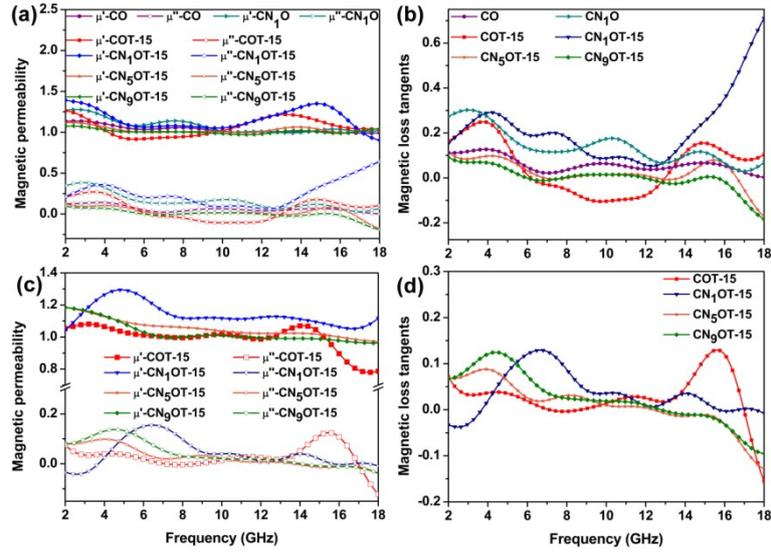
**Fig. S12** Frequency dependence of electromagnetic parameters for various composites, (a) complex permeability and (b) magnetic loss tangent of samples with 20 wt% loading, permeability of (c) CN<sub>1</sub>OT-x with 10 wt% filler content and (d) CN<sub>1</sub>OT-15 with different filler loading.
