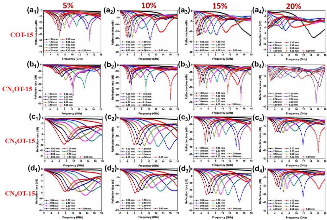
Fig. S10 2D RL curves of the COT and CNOT-x series.
