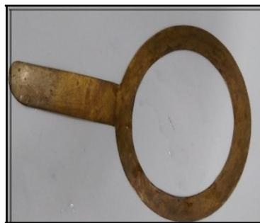
Connector for P- $\text{CeO}_2\text{-CNF/ACF}$  air cathode
