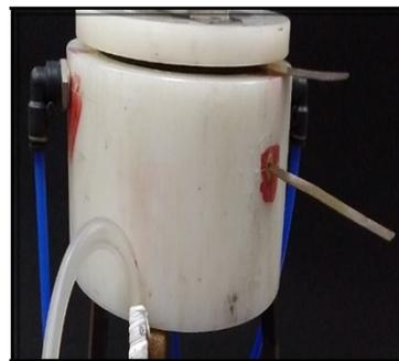
Teflon case which consists anode chamber
