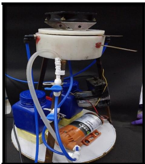
Conical SCMFC front side view
