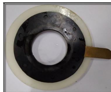
Connector with gasket for holding P- $\text{CeO}_2\text{-CNF/ACF}$  air cathode along with Teflon lid
