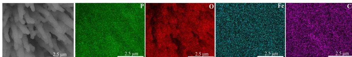
**Figure S10** SEM mapping of Fe-Co-P / NF at a larger range.
