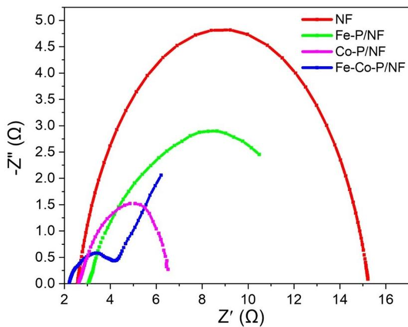
**Figure S5** Electrochemical impedance spectroscopy for bare NF, Fe-Co-P / NF, Co-P / NF, Fe-P / N of HER.
