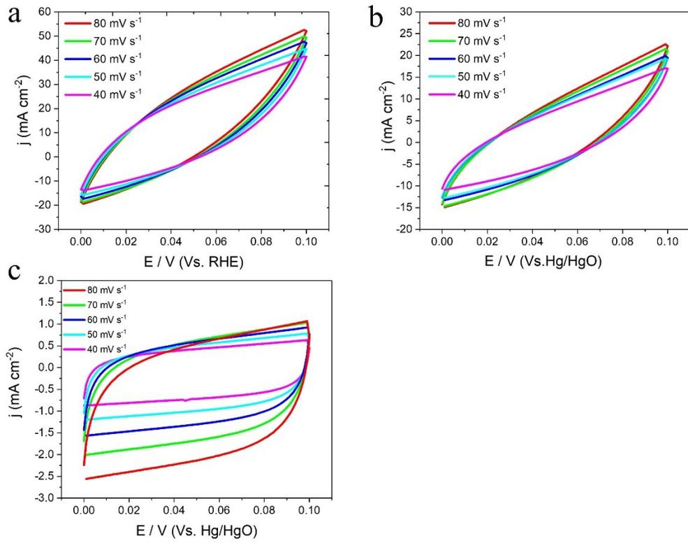
**Figure S3** Cyclic voltammograms of (a) Fe-Co-P/NF (b) Co-P/NF (c) Fe-P/NF.
