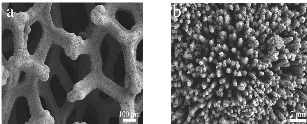
**Figure S6** (a)-(b) SEM imagines of CoCH @ Fe-Co-PBA / NF.
