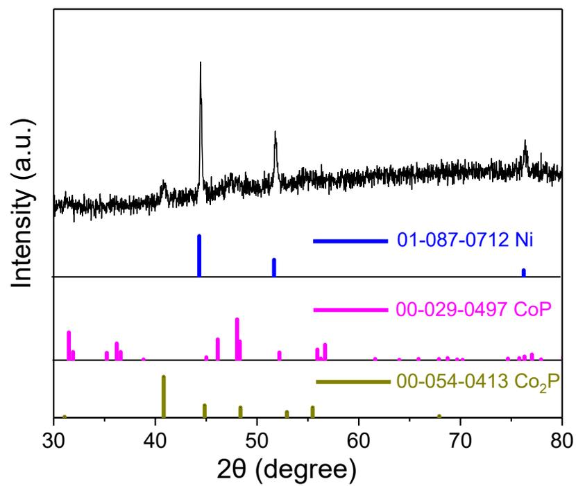
**Figure S9** XRD spectrum of Co-P / NF.
