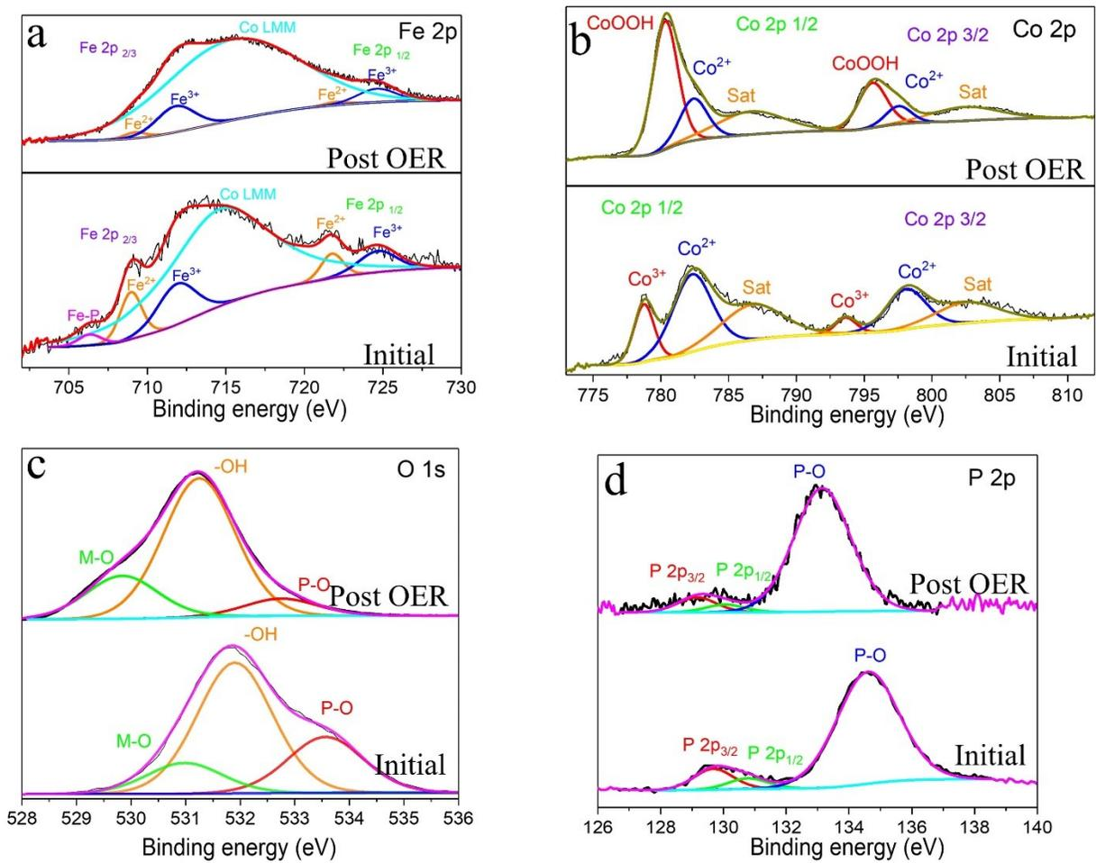
**Figure S4** (a) Fe 2p, (b) Co 2p, (c) O 1s, (d) P 2p of Fe-Co-P / NF spectrums before and after OER test.
