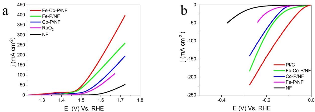
**Figure S15** The pristine polarization curves without  $iR$  correction of the catalysts of (a) HER (b) OER.
