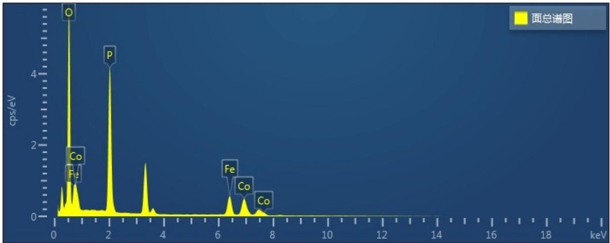
**Figure S8** EDS spectrum of Fe-Co-P / NF.
