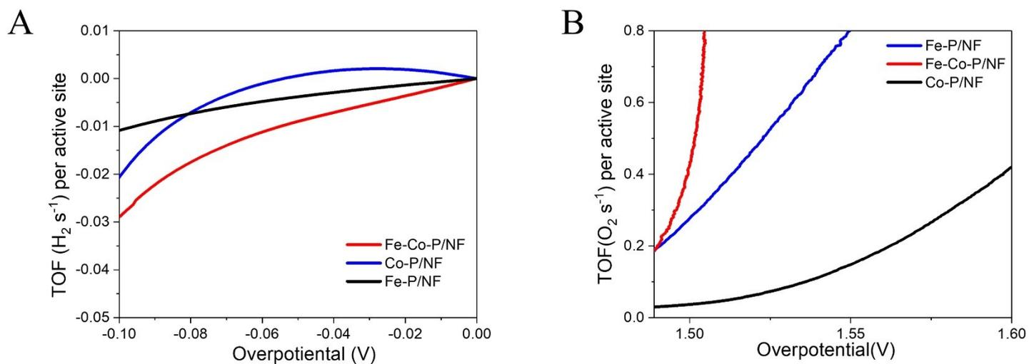
**Figure S13** (a) Calculated  $\text{H}_2$  TOF values for Fe-Co-P/NF, Co-P/NF and Fe-P/NF. (b) Calculated  $\text{O}_2$  TOF values for Fe-Co-P/NF, Co-P/NF and Fe-P/NF.
