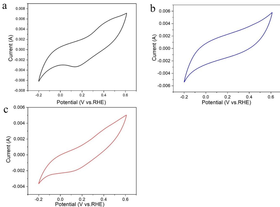
**Figure S12** Cyclic voltammogram (CV) curves of (a) Fe-Co-P/NF (b) Co-P/NF and (c) Fe-P/NF electrocatalysts measured in 1 M PBS (pH = 7) electrolyte at a scan rate of  $50 \text{ mV s}^{-1}$ . Based on the formula of  $n = IV/2Fv$ , the number of active sites was determined to be  $3.23221 \times 10^{-7} \text{ mol}$ ,  $2.55062 \times 10^{-7} \text{ mol}$  and  $1.82949 \times 10^{-7} \text{ mol}$  for Fe-Co-P/NF, Co-P/NF and Fe-P/NF, respectively.
