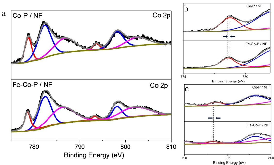
**Figure S2** Co 2p spectrum comparison of Co-P / NF and Fe-Co-P / NF with the partial enlargement pictures.
