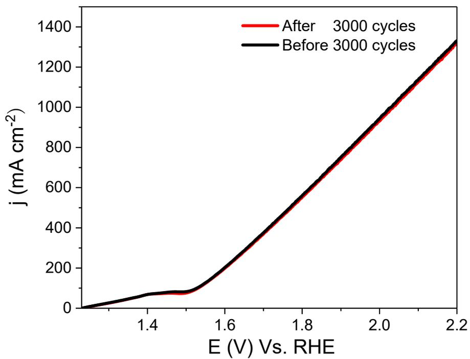
**Figure S11** LSV cruves for Fe-Co-P/NF at high current.
