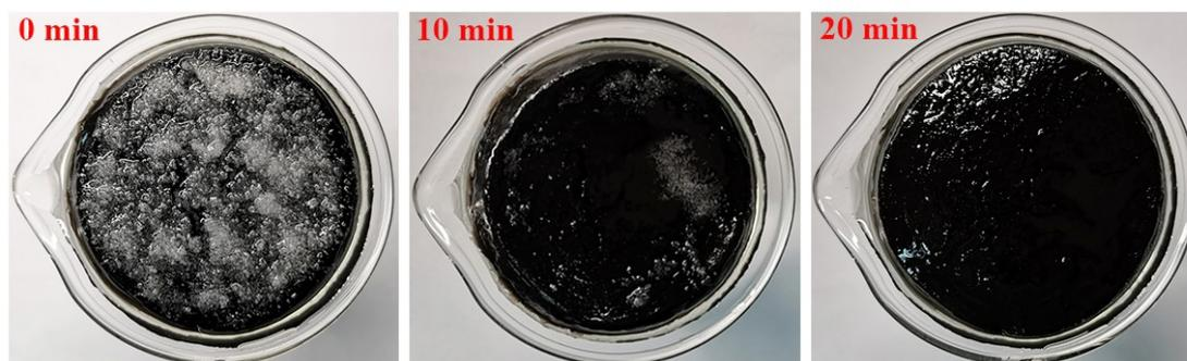
**Fig. S58** The NaCl salt was added on the surface of CPP that was floating on the salty water before exposure to solar irradiation.
