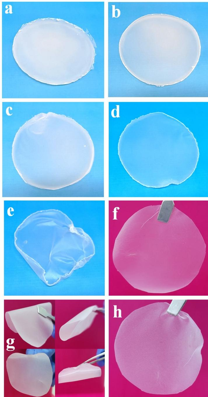
**Fig. S6.** The optical images of YNa-CPEs with different Li-salt content of (a) 10%, (b) 20%, (c) 30%, (d) 35%, and (e) 40%. Illustration of the flexibility and bendability of YNa-CPE-35 (f) before bending, (g) bending at different angles, and (h) returned to initial state after bending.
