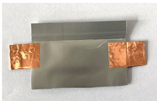
Fig. S13 A digital photo of the soft packaged quasi-solid-state ZHSC.
