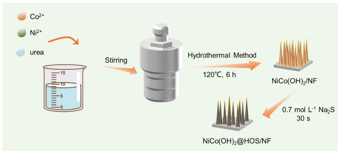
Fig. S1 Schematic illustration of the \text{Ni}_x\text{Co}_{1-x}(\text{OH})_2@\text{HOS}/\text{NF} preparation.
