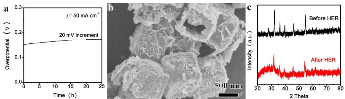
Fig. S17 (a) Chronopotentiometric curves at a constant current density of 50 \text{ mA cm}^{-2} . (b) SEM images of the recovered N-NiS 2 /CoS 2 sample after HER. (c) A comparison of XRD patterns of N-NiS 2 /CoS 2 before and after HER.
