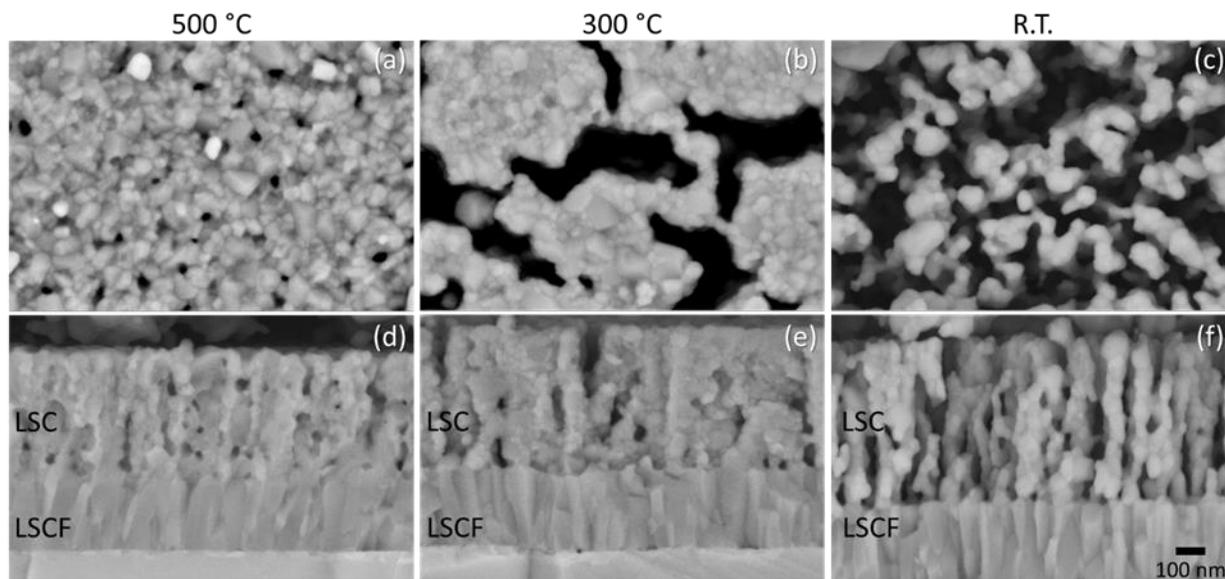
**Fig. S2.** Typical plan-view SEM images of LSC films deposited at (a) 500 °C, (b) 300 °C, and (c) room temperature (R.T.), utilized for symmetrical cells after testing at 700 °C for 300 h in air. (d)-(f): corresponding cross-sectional SEM images.
