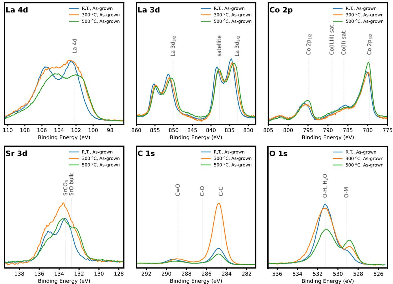
**Fig. S1.** X-ray photoelectron spectra of La 3d, Sr 3d, Co 2p, O 1s core-level spectra of the a) as-grown and b) annealed films prepared at 500 °C, 300 °C, and R.T. Main and satellite peak positions are indicated in each plot.
