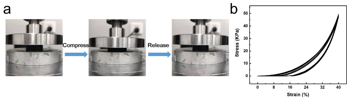
Figure S12. a) Photos of 1.5wt% LPBP hydrogel with compressions with 40% strain. b) Successive compression curves at a strain of 40%.
