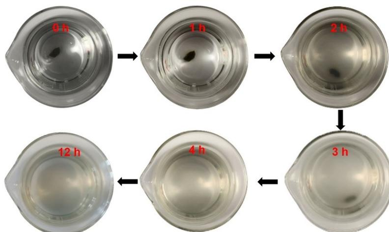
**Figure S29.** Photographs of the degradation of GGOH<sub>0.2</sub> immersed in KOH (1 mol/L) solution at different times.
