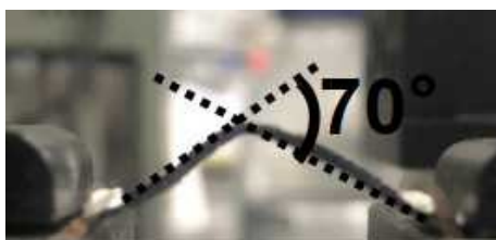
Fig. S4 Digital image of 3DFC@P electrode on cotton showing the bending state at bending angle of 70°.
