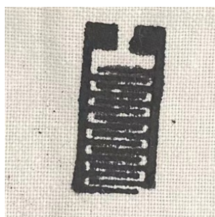
Fig. S3 Digital image of 3DFC@P pattern stencil-printed by mask with finger width of 500 \mu\text{m} and finger spacing of 500 \mu\text{m} .
