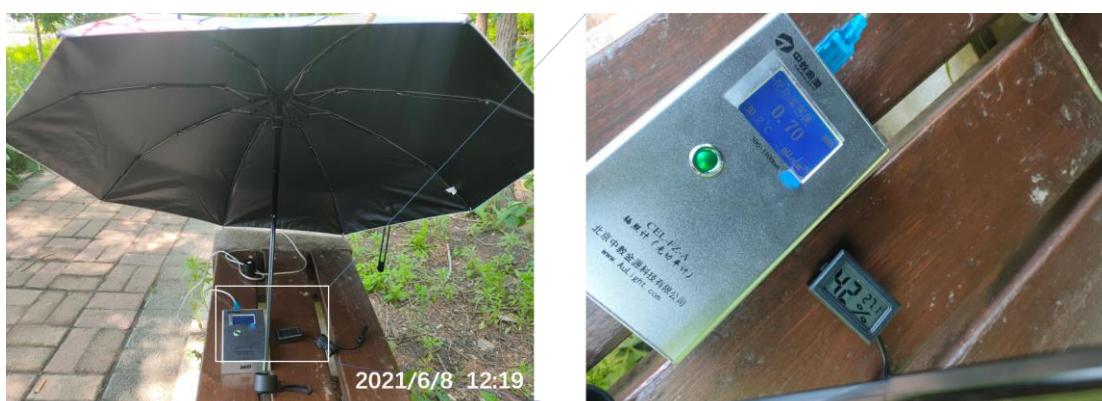
Figure S10 Digital photos of device of outdoor experiments. (The above photo is the desorption process in the sun, and the bottom photo is the sorption process in the shade)
