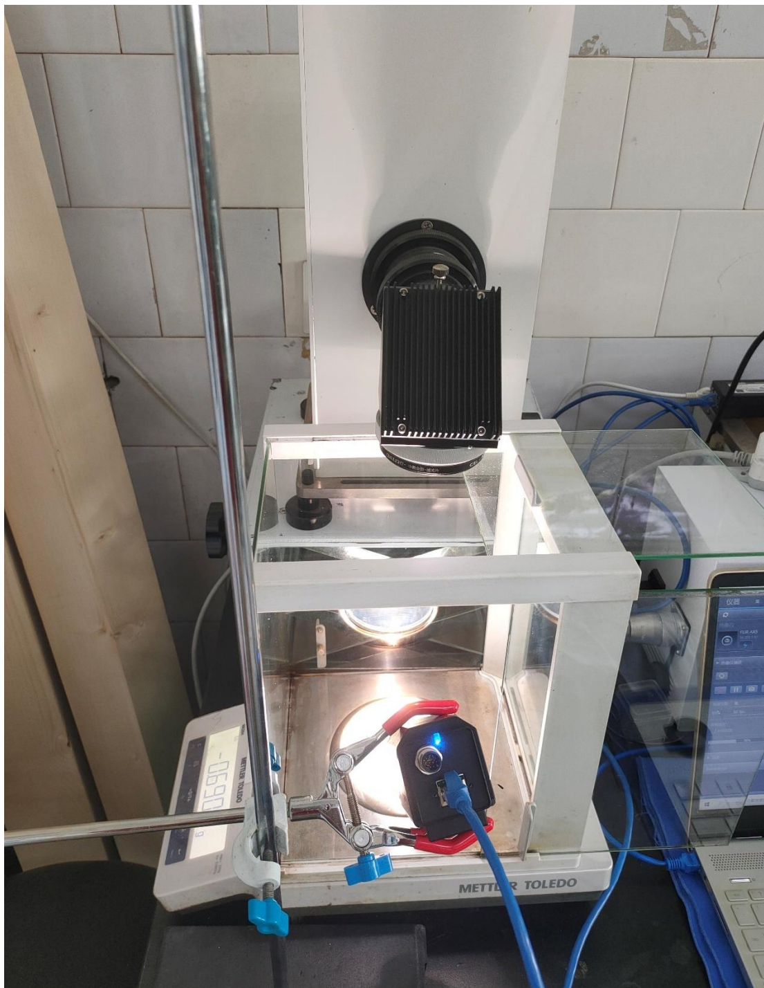
Figure S1 Digital photo of device of indoor solar-powered vapor evaporation.
