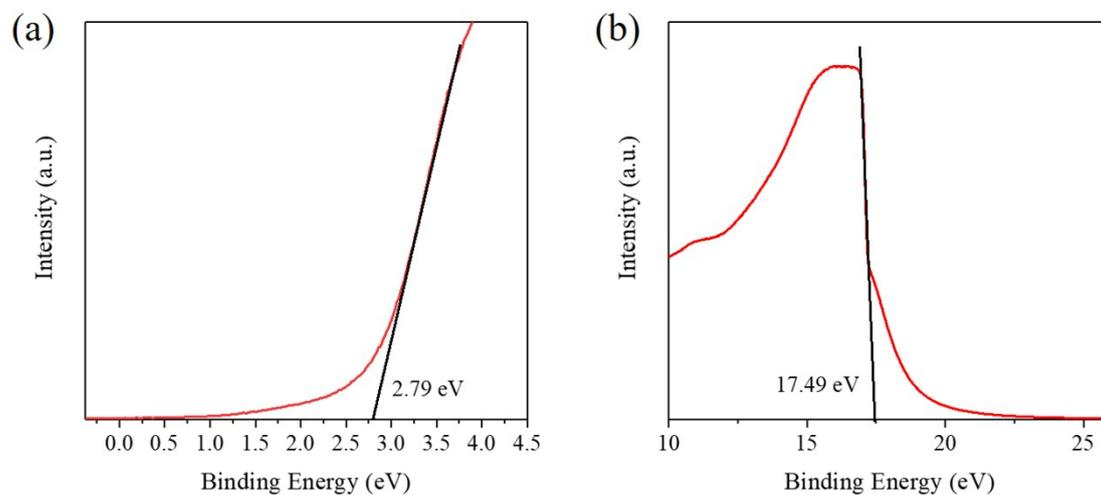
**Figure S5.** a) Near EF region and b) cutoff region of the UPS spectra of 5-SSA/PbI<sub>2</sub> film.
