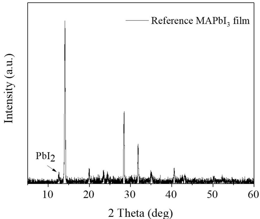
**Figure S4.** XRD pattern of a reference MAPbI<sub>3</sub> film.
