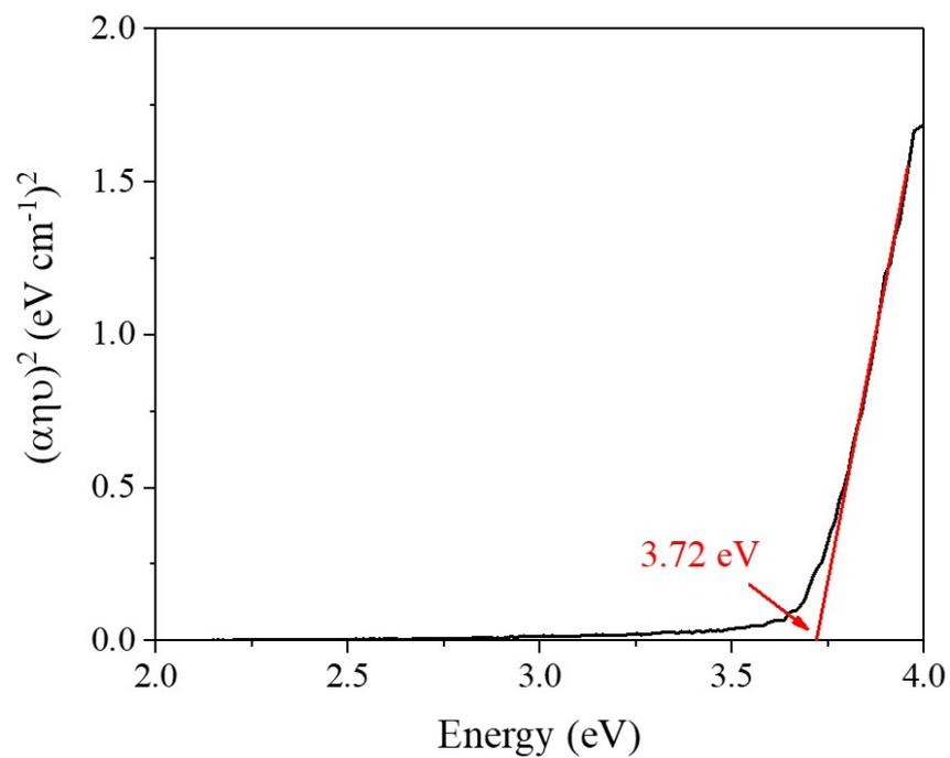
**Figure S6.** The Tauc plot of 5-SSA/PbI<sub>2</sub> film.
