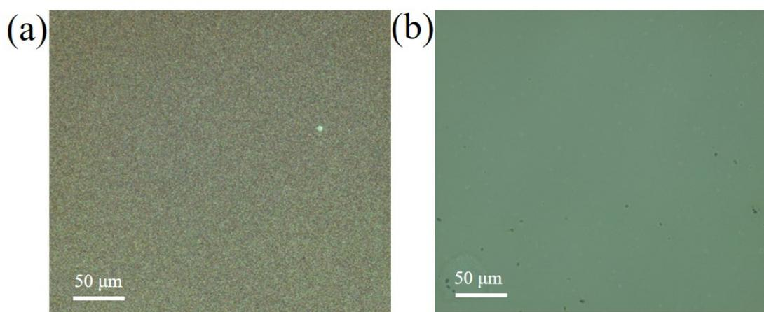
**Figure S1.** Optical microscopy images (a)  $\text{PbI}_2$  and (b) 5-SSA/ $\text{PbI}_2$  films.
