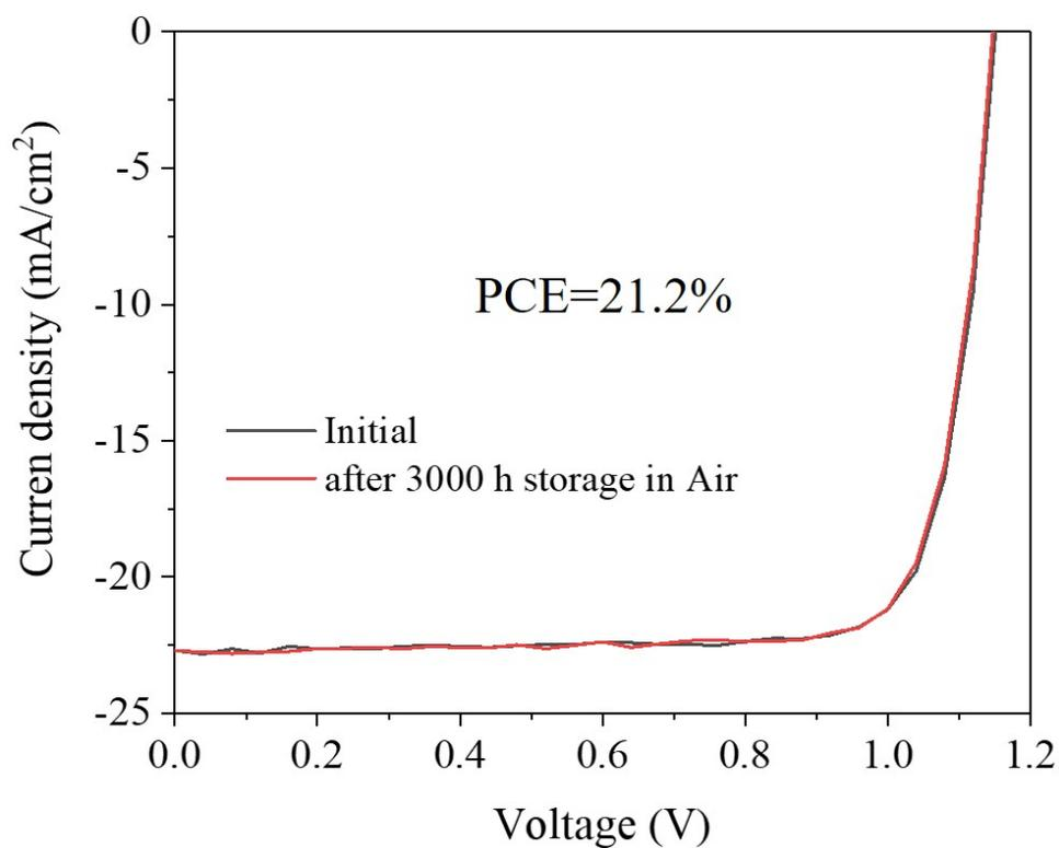
**Figure S9.** The J-V curves of a PSC before and after 3000 hours storage in dark air with 20% humidity.
