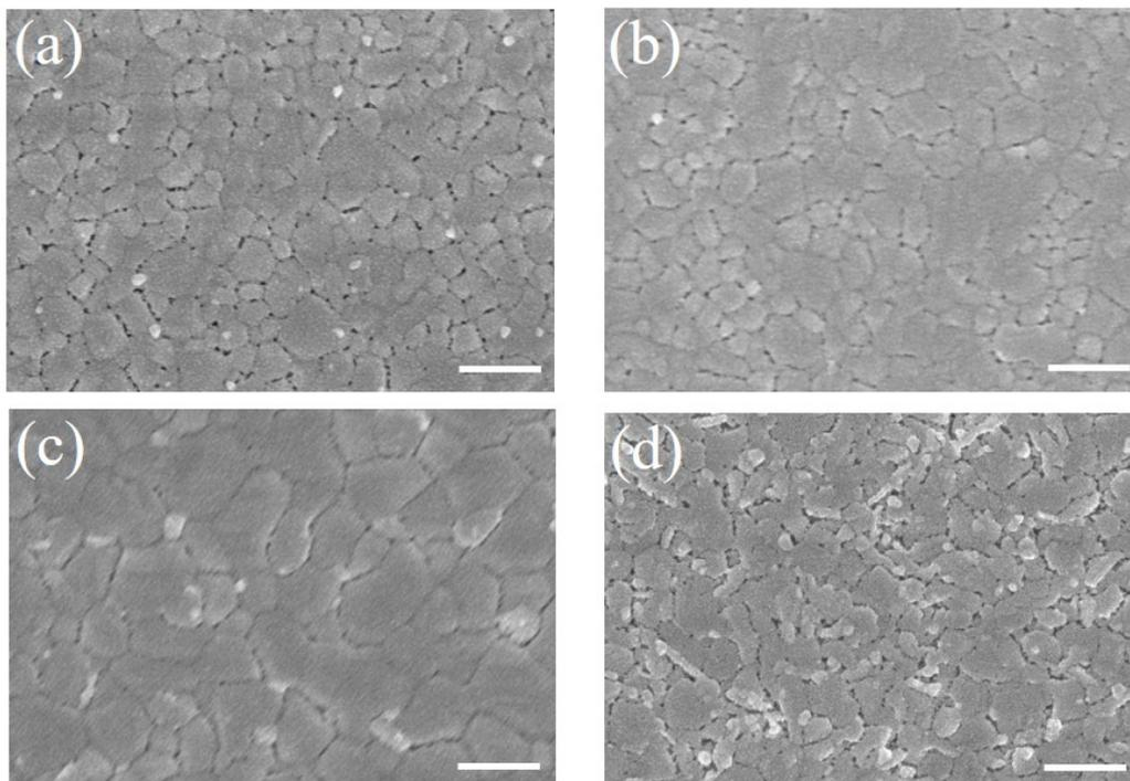
**Figure S2.** Top-view SEM images of MAPbI<sub>3</sub> films with 0 mol% a), 1.0 mol% b), 2.5 mol% c) and 5.0 mol% d) of 5-SSA.
