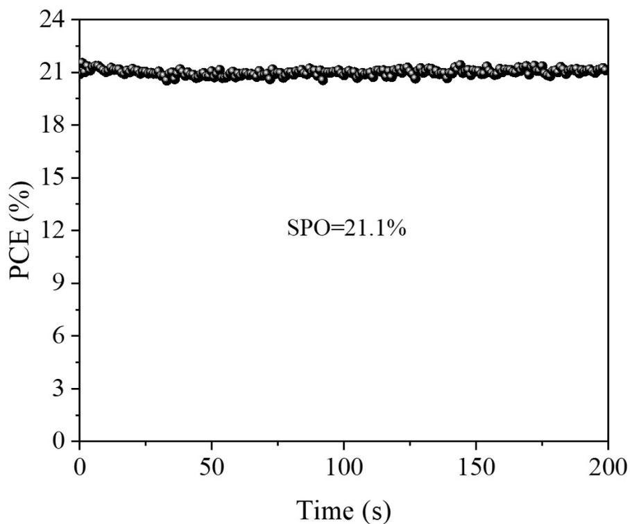
**Figure S8.** The stable power output of a PSC with the 5-SSA/PbI<sub>2</sub> amorphous passivation layer.
