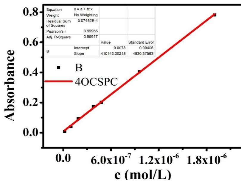
Figure S4. The absorption versus concentration curve of 4OCSPC in THF.
