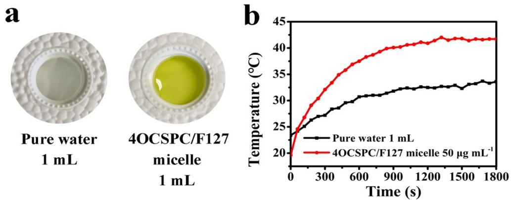
**Figure S5.** (a) Digital photographs of 1 mL pure water and 1 mL  $50 \mu\text{g mL}^{-1}$  4OCSPC/F127 micelles in containers; (b) The temperature changes of 1 mL pure water and 1 mL  $50 \mu\text{g mL}^{-1}$  4OCSPC/F127 micelles under simulated sunlight ( $100 \text{ mW cm}^{-2}$ ).
