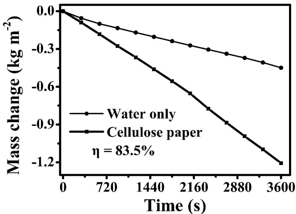
**Figure S10.** Water evaporation curves without (water only) and with cellulose paper-4OCSPC under simulated sunlight with an intensity of  $1 \text{ kW m}^{-2}$  (1 sun). The amount of 4OCSPC used in preparing cellulose paper-4OCSPC is 5 mg. Room temperature is about  $20 \text{ }^{\circ}\text{C}$ .
