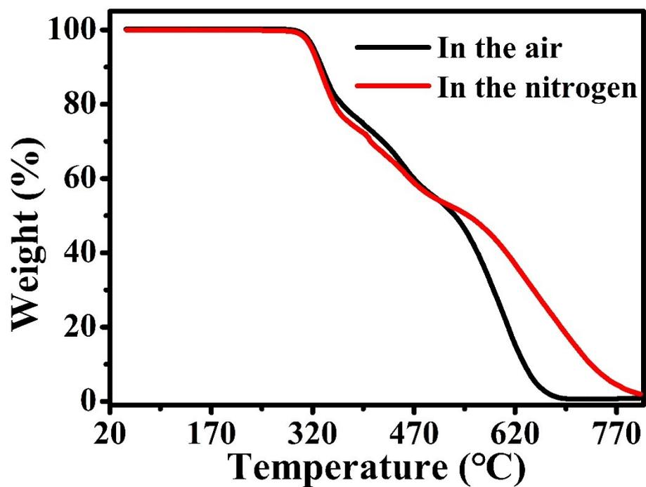
Figure S6. 4OCSPC thermogravimetric of air atmosphere and nitrogen atmosphere.
