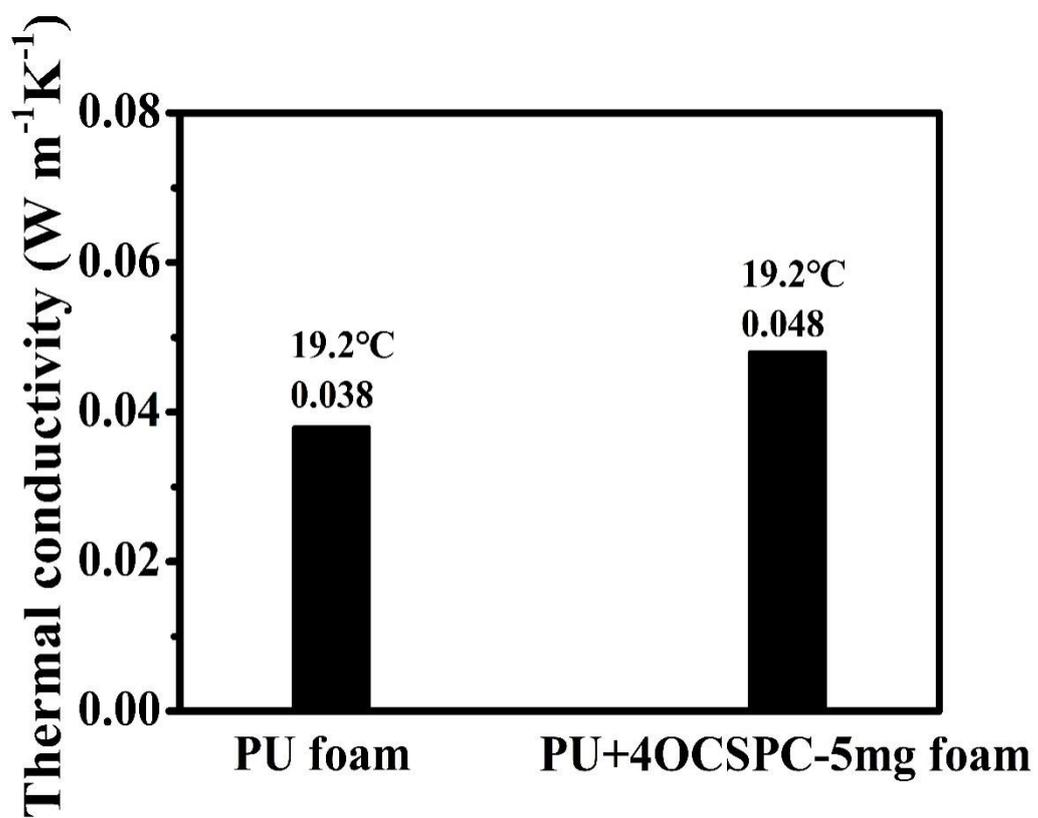
Figure S8. Thermal conductivities of PU and PU+4OCSPC-5 mg foams at 19.2 °C.
