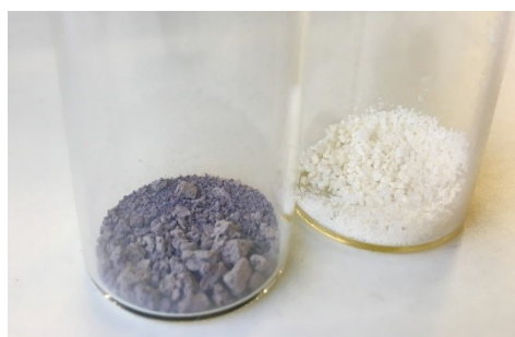
Figure S1. Synthesized off-white porous aromatic framework (PAF-1) and purple sulfonated porous aromatic framework (SPAF).
