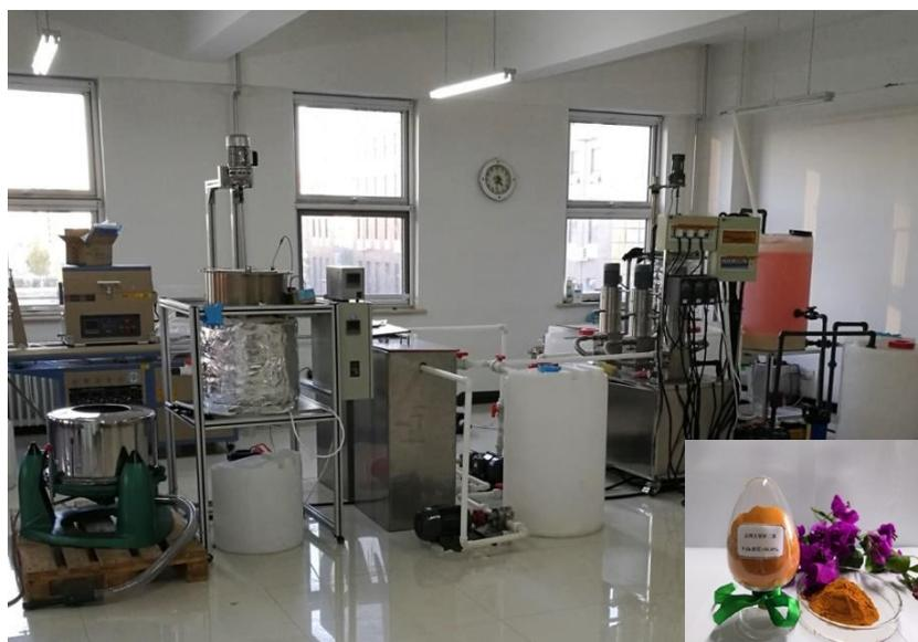
**Figure S1.** Schematic of the pilot-scale production to recover  $\text{V}_2\text{O}_5$  from vanadium-bearing slag, with an optical image of recycled high-purity  $\text{V}_2\text{O}_5$  (labeled as R- $\text{V}_2\text{O}_5$ ).
