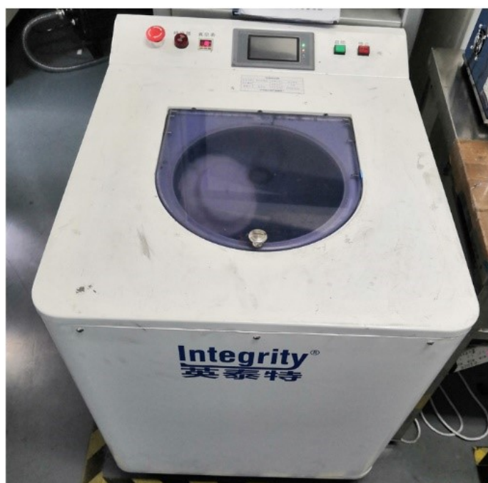
Figure S15. Optical photograph of the planetary rotary homogenizer.
