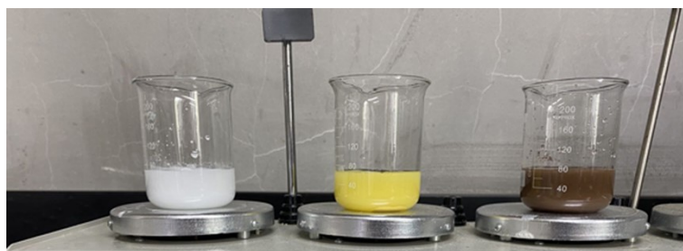
Fig. S20. The digital photos of the as-prepared photocatalysts which were dispersed in water and then placed on a magnetic stirrer for stirring: from left to right were white HD-KPW, yellow ZIS@HD-KPW@ZIS, and brown-black ZIS@HD-KPW@ZIS/AS, respectively.
