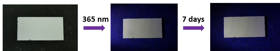
Fig. S26. Photograph of the TLC slide whose surface was written letters N and K and after drying and stand for 7 days at 365 nm light irradiation.
