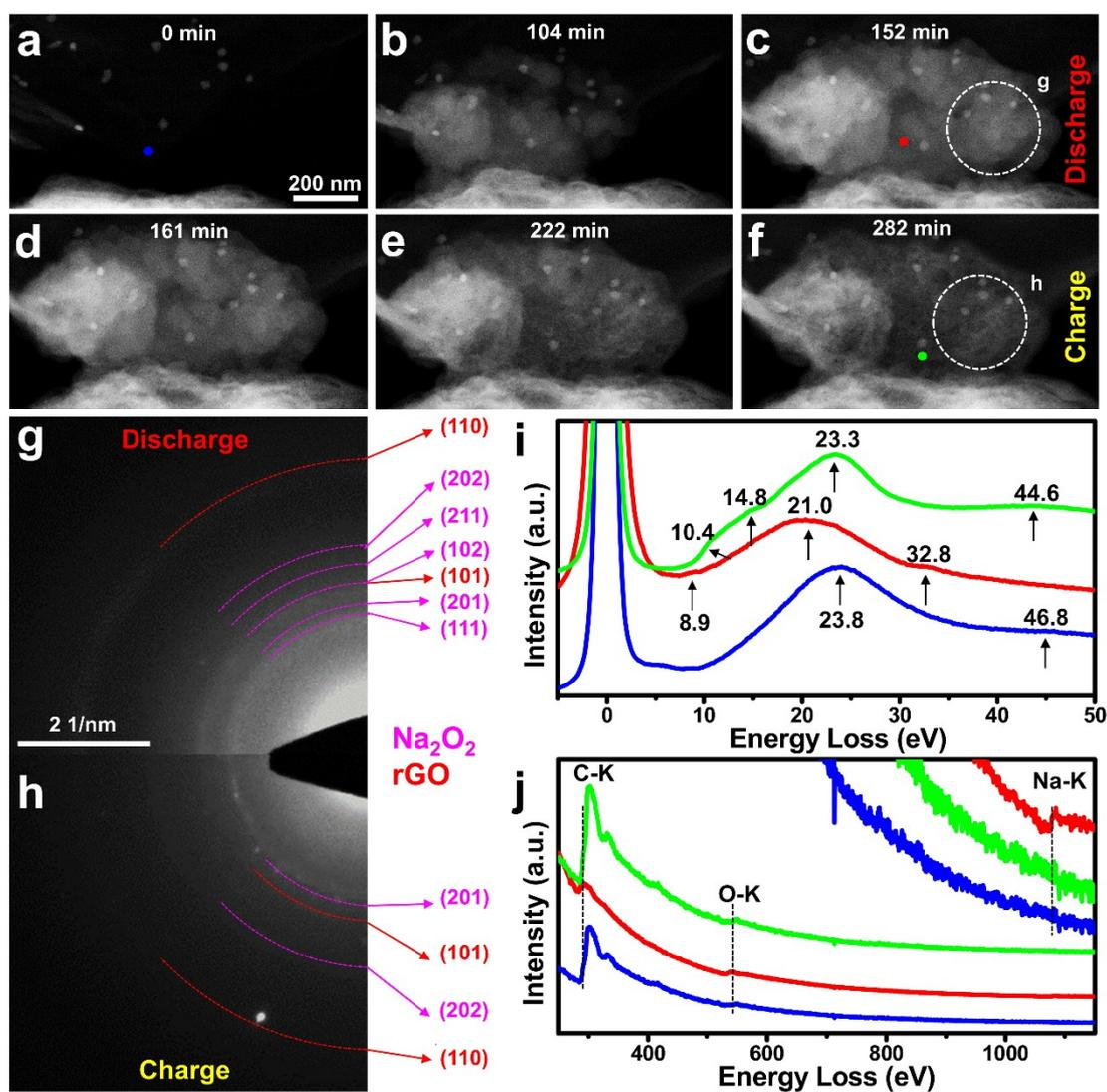
**Fig. S10.** *In situ* TEM observation and characterization of Na-O<sub>2</sub> nanobattery with SA-Co/rGO cathode during the first discharge-charge cycle. (a-f) Time-lapse structure evolution of the SA-Co/rGO cathode in a Na-O<sub>2</sub> nanobattery during the discharge/charge process. (g-h) EDP and (i-j) EELS of the SA-Co/rGO after the discharging and charging processes, respectively.
