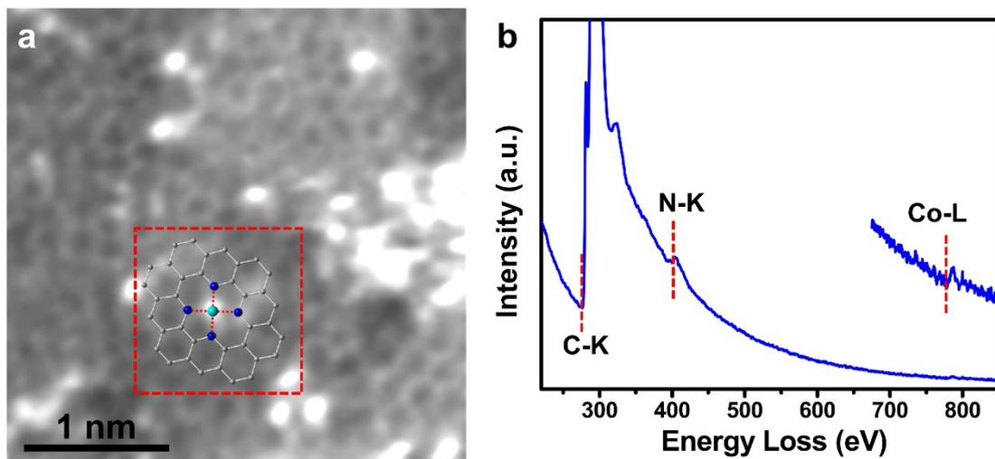
**Fig. S2** (a) ADF image of Co + 4N local structure, (b) Corresponding EELS spectrum taken from the region around individual Co atom.
