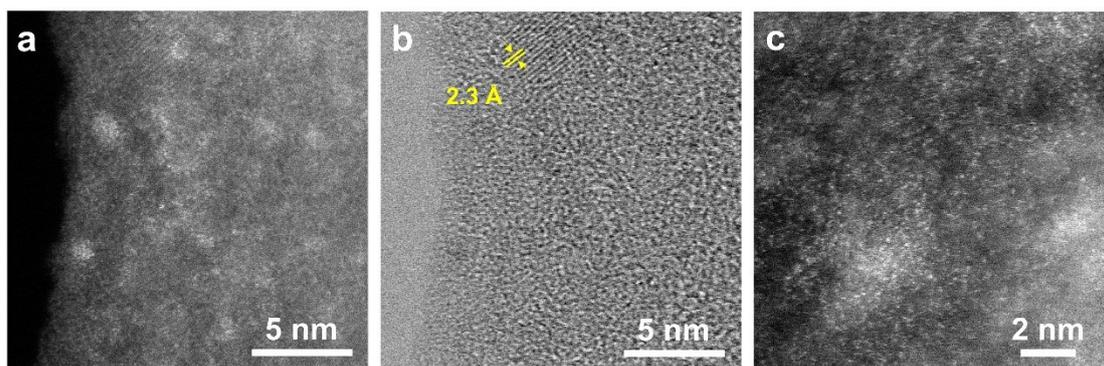
**Fig. S7.** High magnification STEM images of the discharged SA-Co/rGO air cathode. (a) HAADF and (b) ABF images show the fresh formed  $\text{Na}_2\text{O}_2$  lattice. (c) HAADF image shows the single Co atoms.
