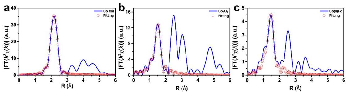
**Fig. S3.** The EXAFS fitting curves at R space. (a) Co foil, (b)  $\text{Co}_3\text{O}_4$  and (c) Co(II)Pc. The Fourier transforms are not corrected for phase shift.
