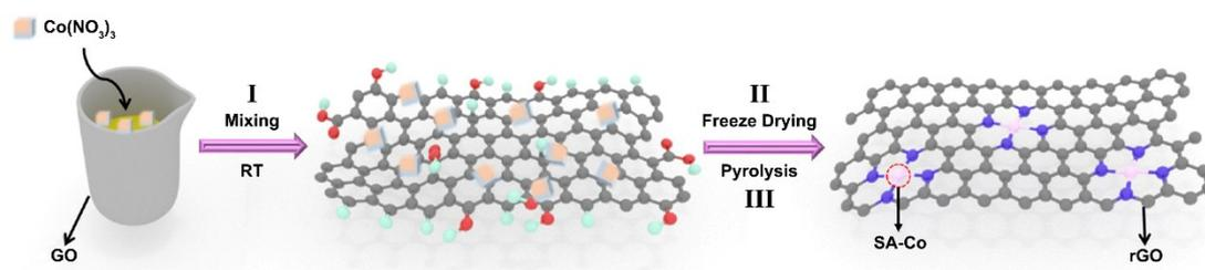
**Fig. S1.** Schematic illustration showing the synthesis process of SA-Co/rGO.
