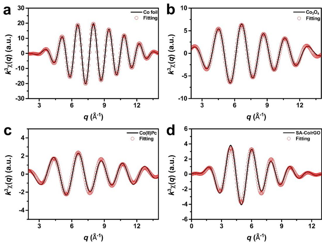
**Fig. S5.** The EXAFS fitting curves at  $q$  space. (a) Co foil, (b)  $\text{Co}_3\text{O}_4$ , (c) Co(II)Pc and (d) SA-Co/rGO.
