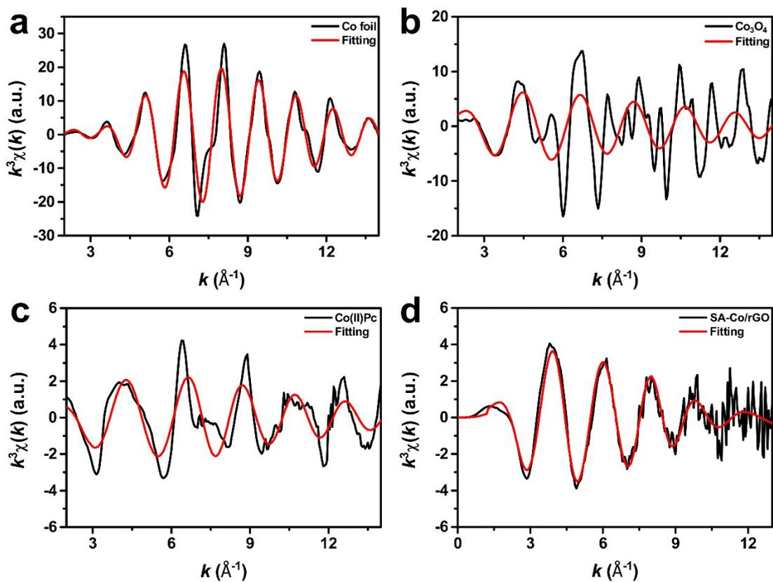
**Fig. S4.** The EXAFS fitting curves at  $k$  space. (a) Co foil, (b)  $\text{Co}_3\text{O}_4$ , (c) Co(II)Pc and (d) SA-Co/rGO.
