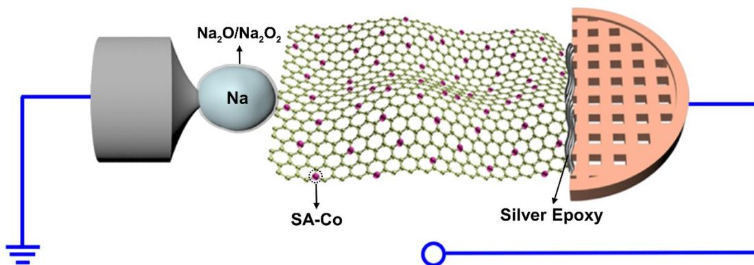
**Fig. S6.** Schematic of the *in situ* experimental setup of a Na-O<sub>2</sub> nanobattery. The nanobattery consists of a SA-Co/rGO cathode, a Na<sub>2</sub>O electrolyte and a Na anode, respectively.
