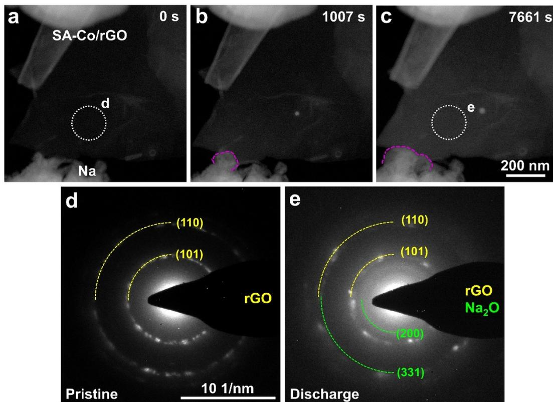
**Fig. S9** *In situ* TEM observation and characterization of a nanobattery in high vacuum condition. (a-c) Time-lapse structure evolution of the SA-Co/rGO cathode during discharging process. (d-e) EDPs of the pristine samples and discharge products on the SA-Co/rGO cathode. White circles mark the locations where EDPs were acquired.
