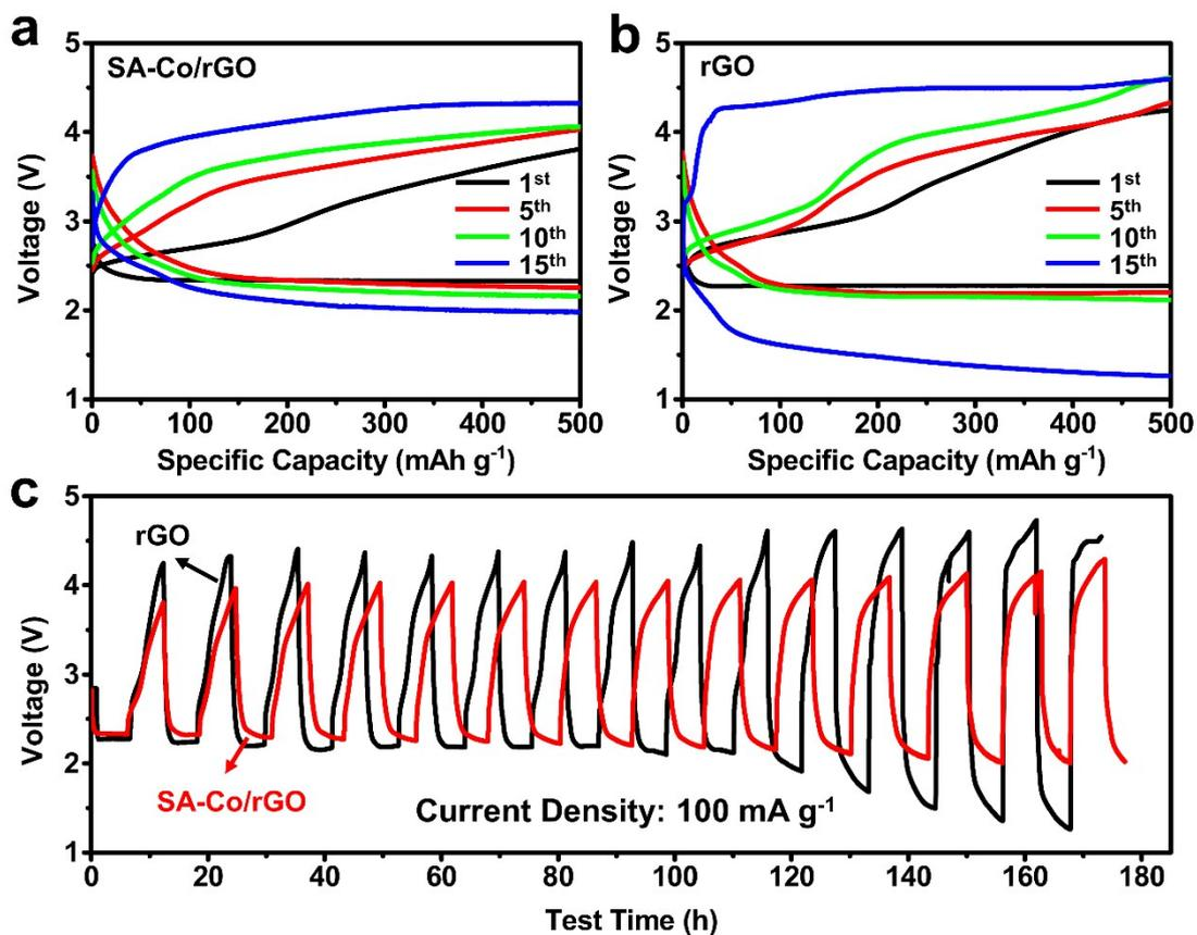
**Fig. S11.** Performance of coin cell Na-O<sub>2</sub> batteries. (a-b) Charge-discharge curves of a coin cell Na-O<sub>2</sub> batteries with SA-Co/rGO cathode and pure graphene cathode, respectively. (c) Cycling stability and terminal discharge/charge voltages of the coin cell Na-O<sub>2</sub> batteries with SA-Co/rGO cathode and pure graphene cathode at a rate of 100 mA g<sup>-1</sup> with a limited specific capacity of 500 mAh g<sup>-1</sup>.
