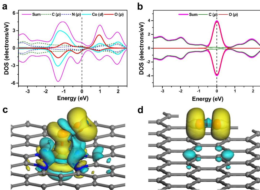
**Fig. S13.** The density of states (DOS) and partial density of states (PDOS): (a) O<sub>2</sub> molecule adsorbed on monolayered SA-Co/rGO surface; (b) O<sub>2</sub> molecule adsorbed on monolayered graphene surface; Isosurface of the difference electron density  $\Delta\rho$  for O<sub>2</sub> adsorbed on: (c) monolayered SA-Co/rGO surface; (d) monolayered graphene surface. (yellow for  $\Delta\rho > 0$  and blue for  $\Delta\rho < 0$ )
