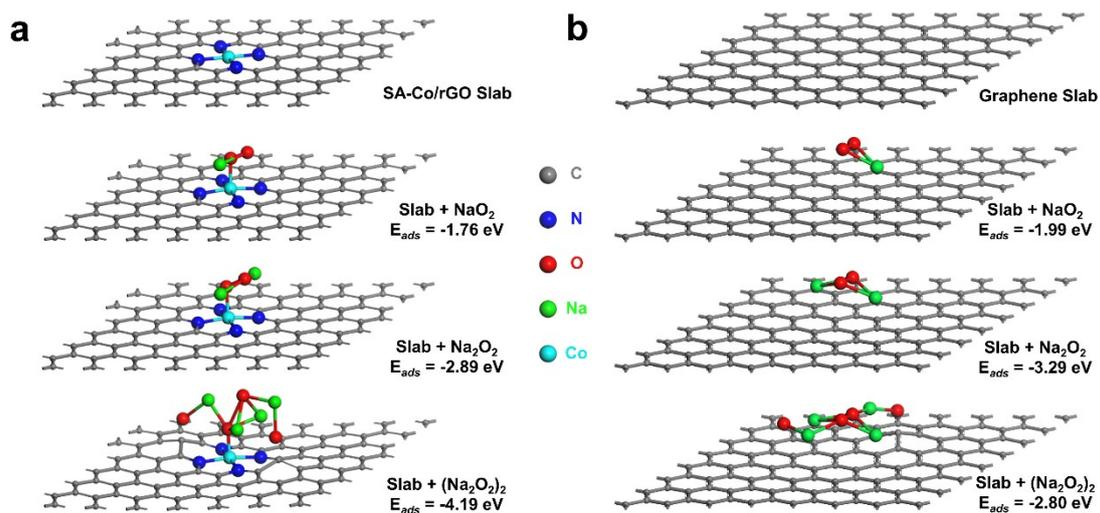
**Fig. S14.** Side view of the optimized structures corresponding to the diagrams for the discharge-charge reactions. (a) monolayered SA-Co/rGO; (b) monolayered graphene.
