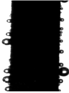
146 Fig. S6. Gas bubble on the static \text{TiO}_2\text{-OV@Ti-F} anode observed by camera (AFT- 147 ZL0920). Conditions: [\text{Na}_2\text{SO}_4] = 50 \text{ mM} and current density = 25 \text{ mA cm}^{-2} .
