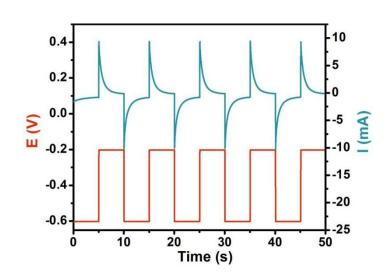
81 Fig. S1 I-V curves of square wave pulse method for anchoring Au atoms on OVs-
