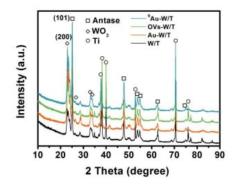
Fig. S2 XRD spectra of W/T, Au-W/T, OVs-W/T and <sup>S</sup>Au-W/T. For both W/T, <sup>S</sup>Au-W/T and <sup>S</sup>Au-T/W composites, besides characteristic diffraction peaks of anatase
