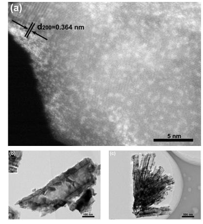
109 Fig. S4 (a) HAADF-STEM image and (b) (c) STEM image of Au-W/T. Au was
