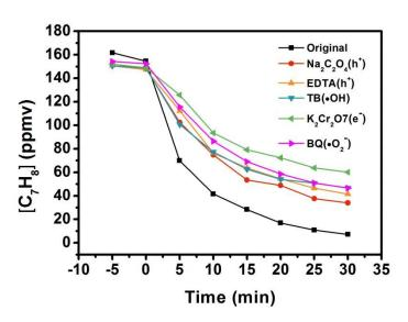
Fig. S6 Quenching experiment over <sup>S</sup>Au-W/T. the quenchers were loaded on suface
