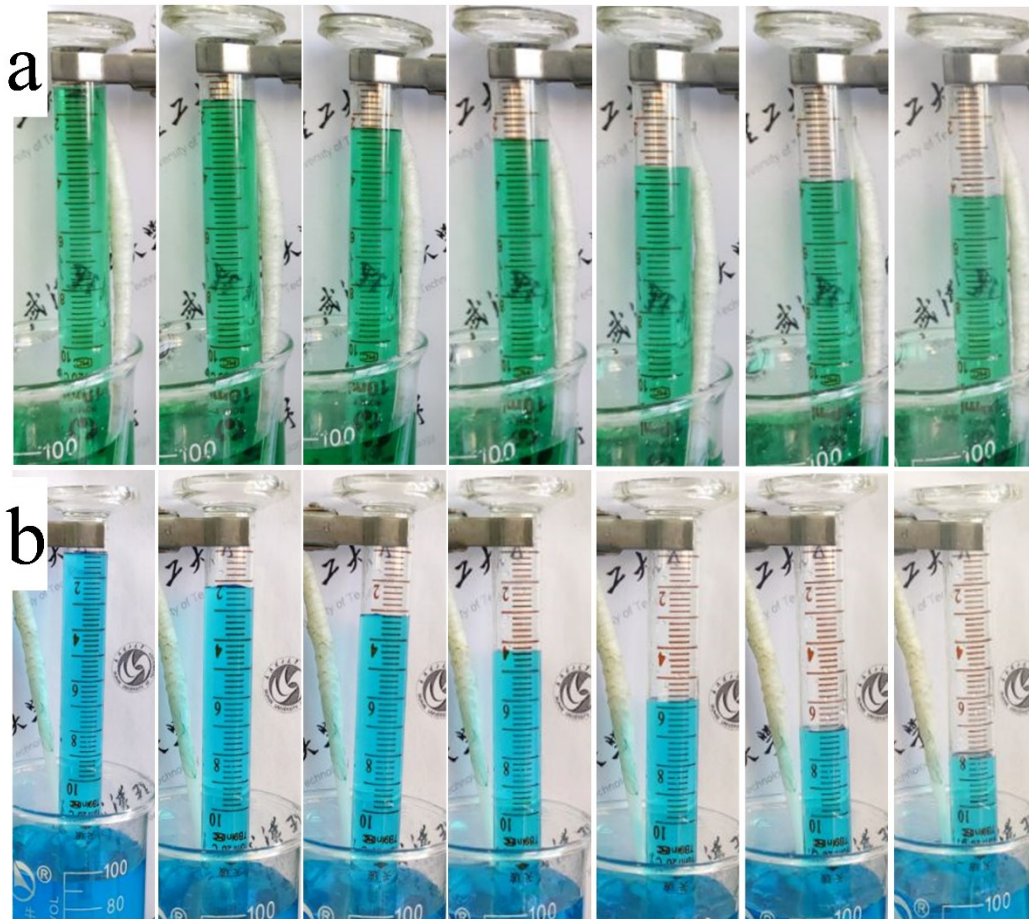
Figure S11. (a-b) Changes in the volume of (a) O_2 and (b) H_2 over time.
