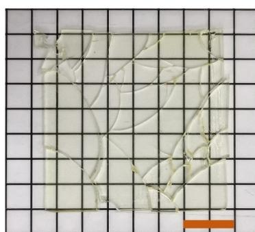
**Fig. S3.** The extremely fragile sample of P-HEA-co-HEMA with 80 mol% of hard HEMA monomer (scale bar, 1 cm).
