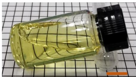
**Fig. S5.** The clear nutrients PTS are stable after being stored in a light-free condition (testing time: 90 days, scale bar, 1 cm).
