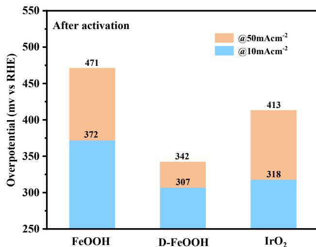
**Figure S1.** The comparison of overpotential under current density of 10 and 50 mA cm<sup>-2</sup> for FeOOH and D-FeOOH catalysts after OER activation, along with the benchmark IrO<sub>2</sub> reference.
