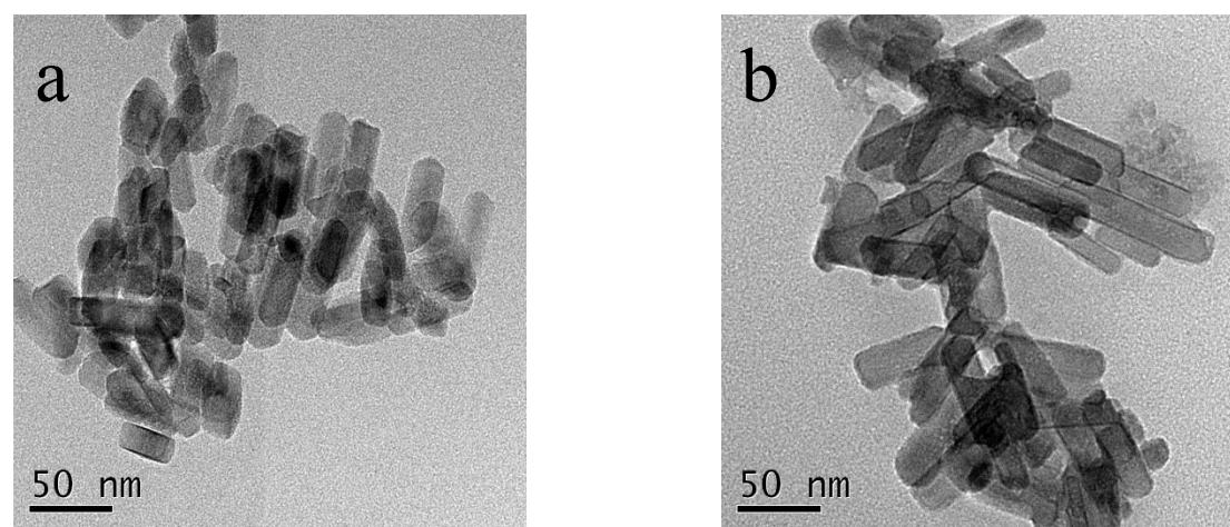
**Figure S4.** TEM of the FeOOH a) and D-FeOOH b) after OER activation.
