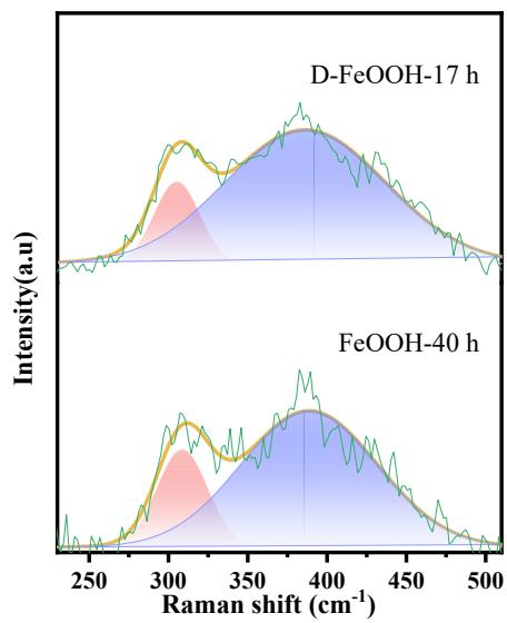
**Figure S9.** Fit curves of partial in-situ Raman spectra of D-FeOOH-17 h and FeOOH-40 h.
