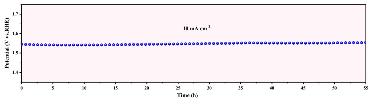
**Figure S2.** Chronopotentiometric curve of long-term stability for D-FeOOH after activation in 1 M KOH electrolyte at a current density of 10 mA cm<sup>-2</sup>.
