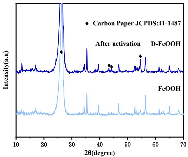
**Figure S5.** XRD pattern of the FeOOH and D-FeOOH after OER activation.
