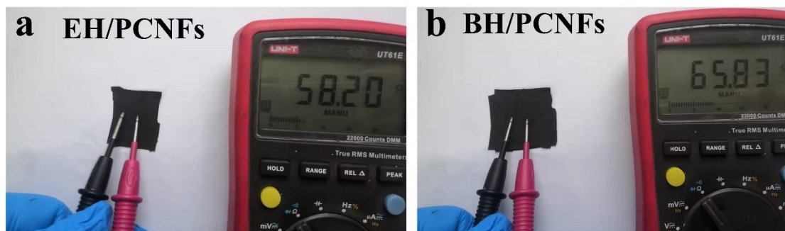
Fig. S7. the conductivity values of the prepared two electrodes. (a) EH/PCNFs; (b) BH/PCNFs.
