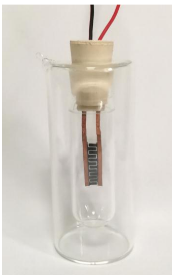
Fig. S17 Optical image of the low-temperature testing equipment (the ST-MSC placed and sealed in a homemade double-layer quartz container).
