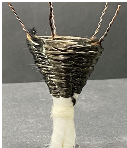
Fig. S10. Optical image of 3D CFC-Cone without upper cotton rods.
