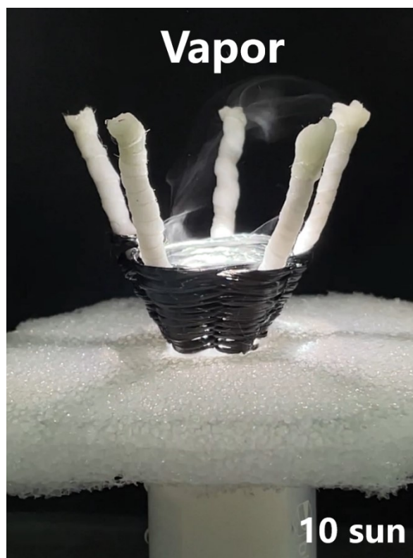
Fig. S9. Optical image of vapor generating from CFC-Cone-5.
