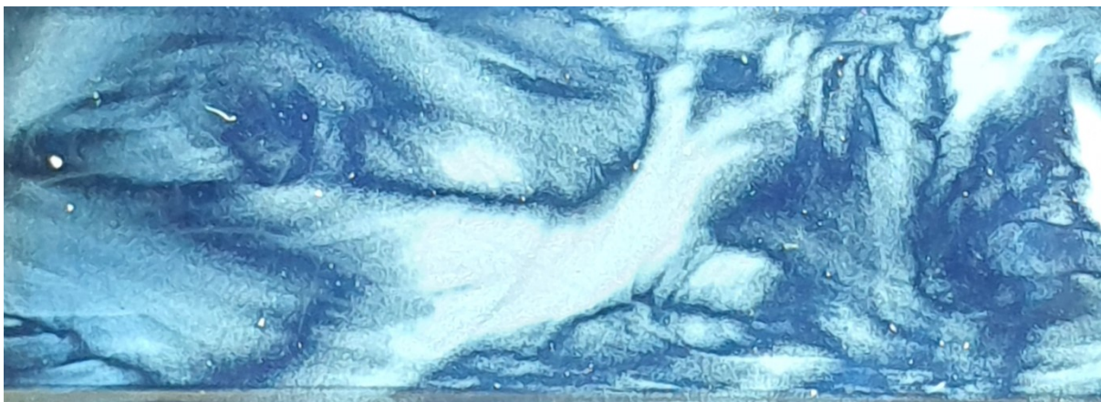
Fig. S4. Polarized optical micrograph of GO dispersion. The gigantic aspect ratio of our as-prepared amphiphilic GO sheets facilitate the formation of liquid crystals at concentrations as low as 0.1 g/L.
