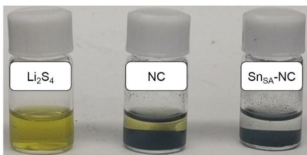
**Figure S11.** The digital photograph of  $\text{Li}_2\text{S}_4$  solutions after exposure to NC and  $\text{Sn}_{\text{SA}}\text{-NC}$ .
