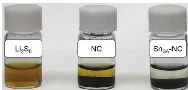
**Figure S10.** The digital photograph of Li<sub>2</sub>S<sub>8</sub> solutions after exposure to NC and Sn<sub>SA</sub>-NC.
