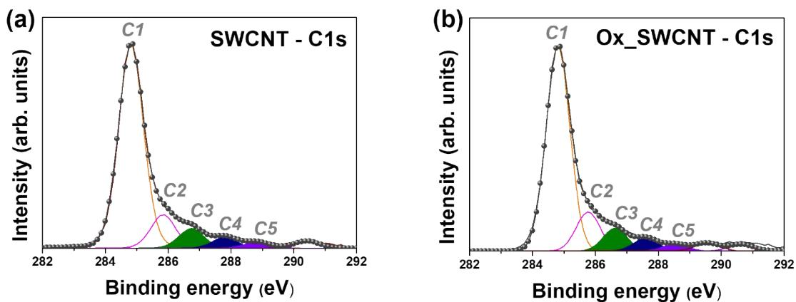
**Figure S7.** Deconvolution of high-resolution C1s X-ray photoelectron spectroscopy profiles of (a) SWCNT and (b) Ox-SWCNT buckypaper.
