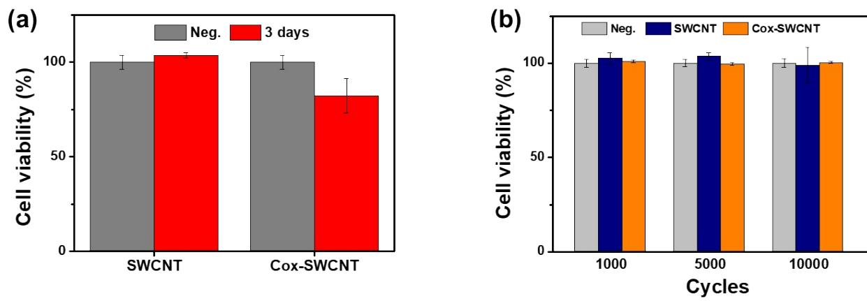
**Figure S2.** (a) Cell viability of human fibroblast cells measured using MTT assays after 3 days of exposure to SWCNT and Cox-SWCNT buckypaper electrodes. (b) Cell viability of human fibroblast cells measured using MTT assays after cyclic voltammetry from 1,000 to 10,000 cycles.
