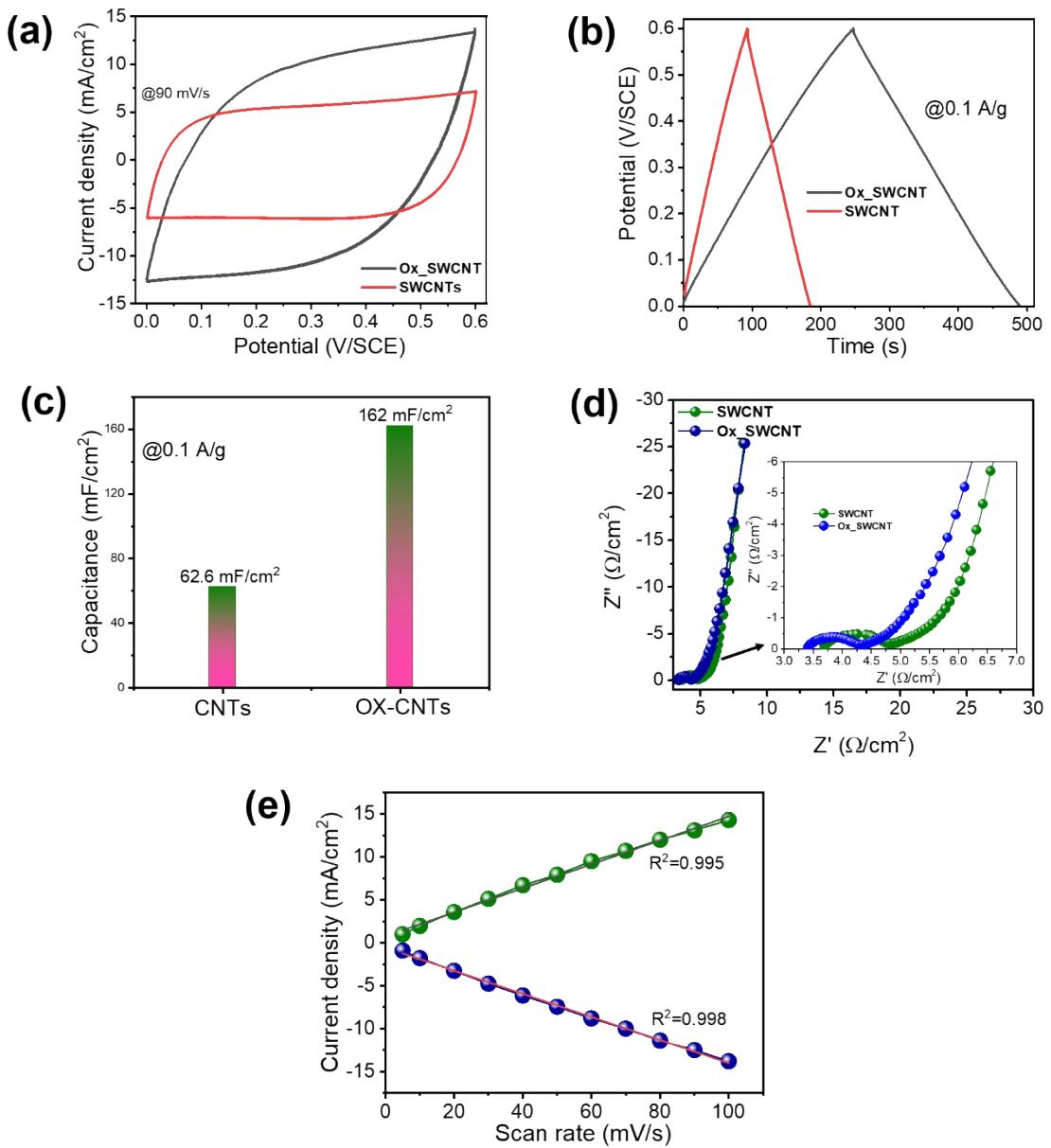
**Figure S5.** Three-electrode cell data; (a) cyclic voltammetry curves of SWCNT and Ox-SWCNT electrodes at a scan rate = 90 mV·s<sup>-1</sup> tested in simulated body fluid. (b) Galvanostatic charge-discharge profiles and (c) capacitance of SWCNT and Ox-SWCNT at 0.1A/g. (d) Nyquist plot and (e) plot of cathodic and anodic current at various scan rates.
