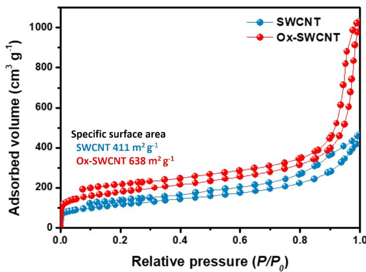
**Figure S8.** N<sub>2</sub> adsorption-desorption curves of SWCNT and Ox-SWCNT.
