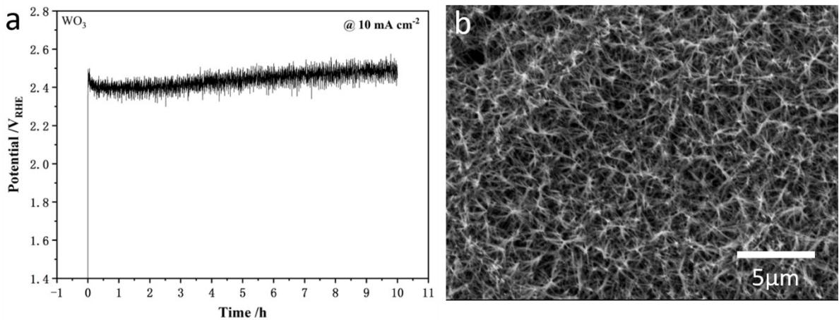
**Fig. S10.** Stability of pure WO<sub>3</sub>. (a) Test of at 10 mA cm<sup>-2</sup>, (b) the decayed morphology in SEM image.
