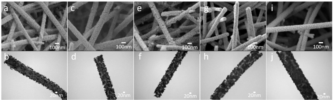
**Fig. S3.** Surface Ir/Ru ratio depended morphologies of (a-b) Ir<sub>1.7</sub>Ru<sub>0.9</sub>@WO<sub>3</sub>, (c-d) Ir<sub>3.5</sub>Ru<sub>1</sub>@WO<sub>3</sub>, (e-f) Ir<sub>4.5</sub>Ru<sub>1</sub>@WO<sub>3</sub>, (g-h) Ir<sub>3.2</sub>Ru<sub>1.6</sub>@WO<sub>3</sub>, (i-j) Ir<sub>3.2</sub>Ru<sub>1.6</sub>@WO<sub>3</sub>.
