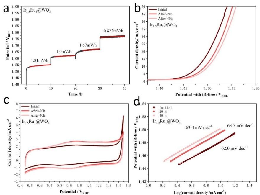
**Fig. S6.** The performance of  $\text{Ir}_{3.5}\text{Ru}_1@\text{WO}_3$  during the stability operation tested in 0.5 M  $\text{N}_2$ -saturated  $\text{H}_2\text{SO}_4$  at 30 °C. (a) Step chronopotentiometry operation at 10, 30, 50, 100  $\text{mA cm}^{-2}$  for each step. (b) LSV curves, (c) CV curves, (d) Tafel curves at initial, after 20 h and 40 h operation.
