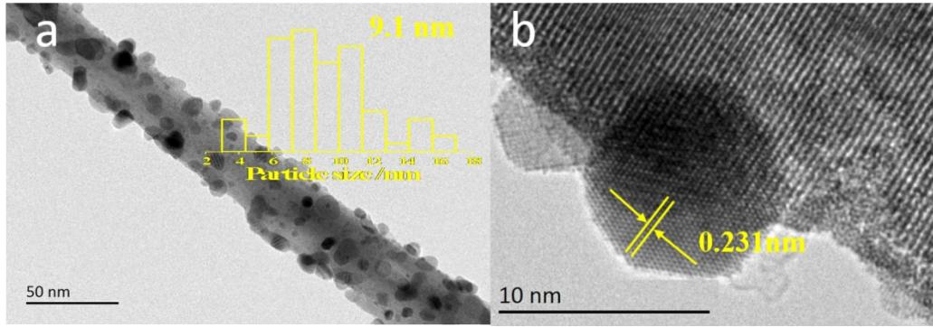
**Fig. S2.** Intermediate Ru@WO<sub>3</sub> TEM images. (a) Overall morphology of the nanorod with Ru seed size. (b) Locality morphology on Ru seed marked with interplanar spacing.
