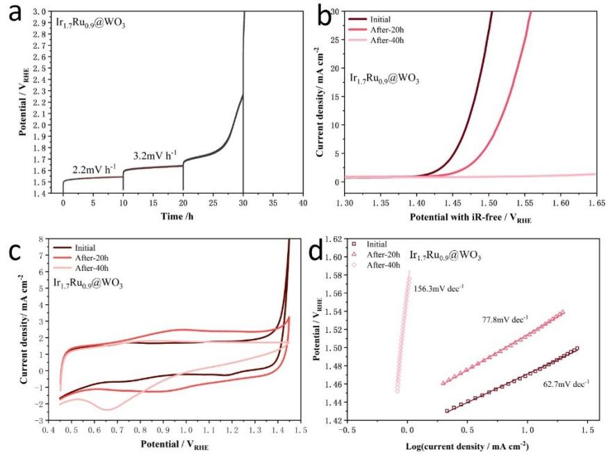
**Fig. S7.** Performance of  $\text{Ir}_{1.7}\text{Ru}_{0.9}@\text{WO}_3$  during the stability operation tested in 0.5 M  $\text{N}_2$ -saturated  $\text{H}_2\text{SO}_4$  at 30 °C. (a) Step chronopotentiometry operation at 10, 30, 50, 100  $\text{mA cm}^{-2}$  for each step. (b) LSV curves, (c) CV curves, (d) Tafel curves at initial, after 10 h, 20 h, 30 h and 40 h operation.
