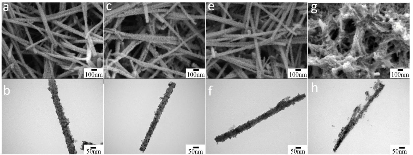
**Fig. S9.** Decayed morphologies of IrR@WO<sub>3</sub> annealed in (a-b) 400 °C, (c-d) 500 °C, (e-f) 600 °C, (g-h) 700 °C after operation.
