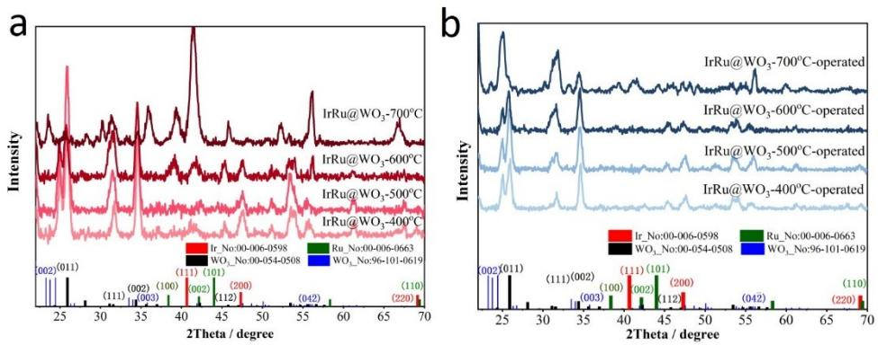
**Fig. S12.** XRD result of IrRu@WO<sub>3</sub> annealed in 400~700°C before (a) after (b) the step chronopotentiometry operation.
