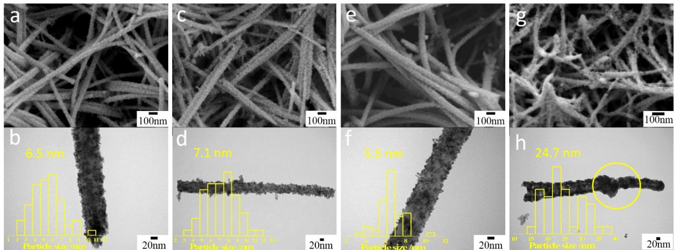
**Fig. S5.** Temperature depended morphologies of  $\text{Ir}_{3.5}\text{Ru}_1@\text{WO}_3$  annealed in (a-b) 400 °C, (c-d) 500 °C, (e-f) 600 °C, (g-h) 700 °C.
