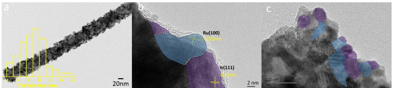
**Fig. S14.** TEM morphologies of IrRu@WO<sub>3</sub> after the stability operation. (a) Overall morphology of the nanorod with coating particle size. (b~c) Locality morphology with distinguished lattice figure marked by colored in blue (Ru) and purple (Ir).
