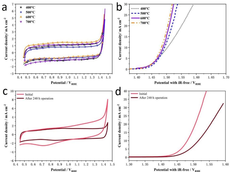
**Fig. S11.** OER performances of IrRu@WO<sub>3</sub> accompanying with annealing temperature 400~700°C, (a) CV and (b) LSV. (c)
