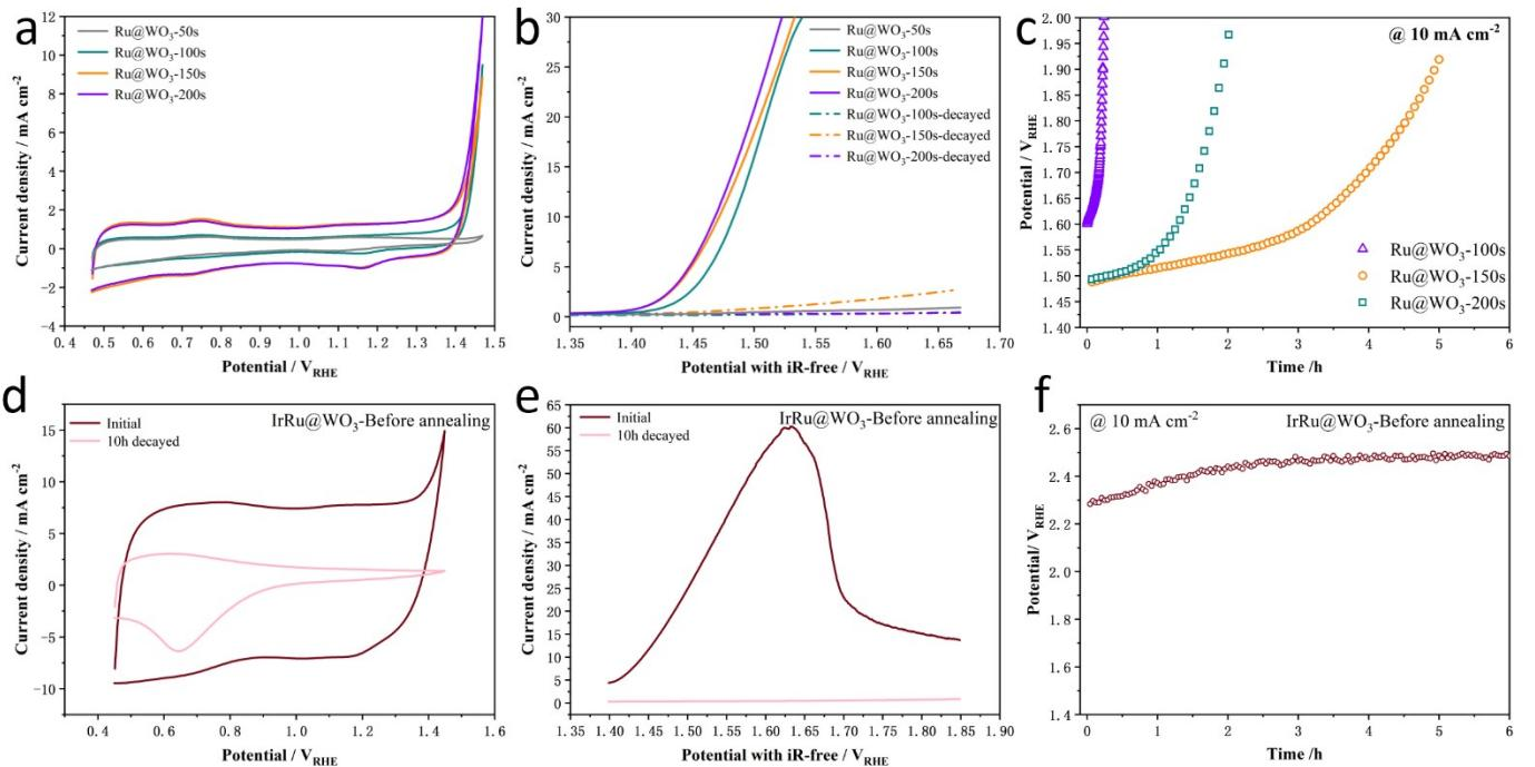
**Fig. S8.** OER performances for (a) CV curves, (b) LSV curves, (c) stability curves at 10  $\text{mA cm}^{-2}$  of  $\text{Ru}@\text{WO}_3$ -600 °C with different deposition time; (d) CV curves, (e) LSV curves, (f) stability curves at 10  $\text{mA cm}^{-2}$  of  $\text{IrRu}@\text{WO}_3$  without annealing in 30 °C, 0.5 M  $\text{N}_2$ -saturated  $\text{H}_2\text{SO}_4$ .
