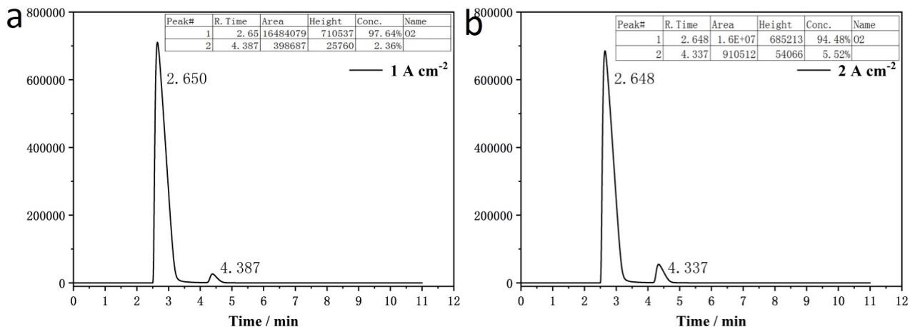
**Fig. S18** Online GC result of the O<sub>2</sub> concentration in the anode gas at (a) 1.0 A cm<sup>-2</sup> and (b) 2.0 A cm<sup>-2</sup>.
