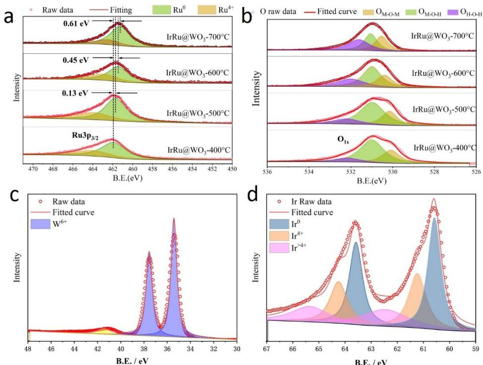
**Fig. S4.** Supplemental XPS result of IrRu@WO<sub>3</sub>-400-700°C (a) Ru3p (b) O1s, (c) W4f of pure WO<sub>3</sub> and (d) Ir4f of commercial Ir Black(JM) spectrogram.
