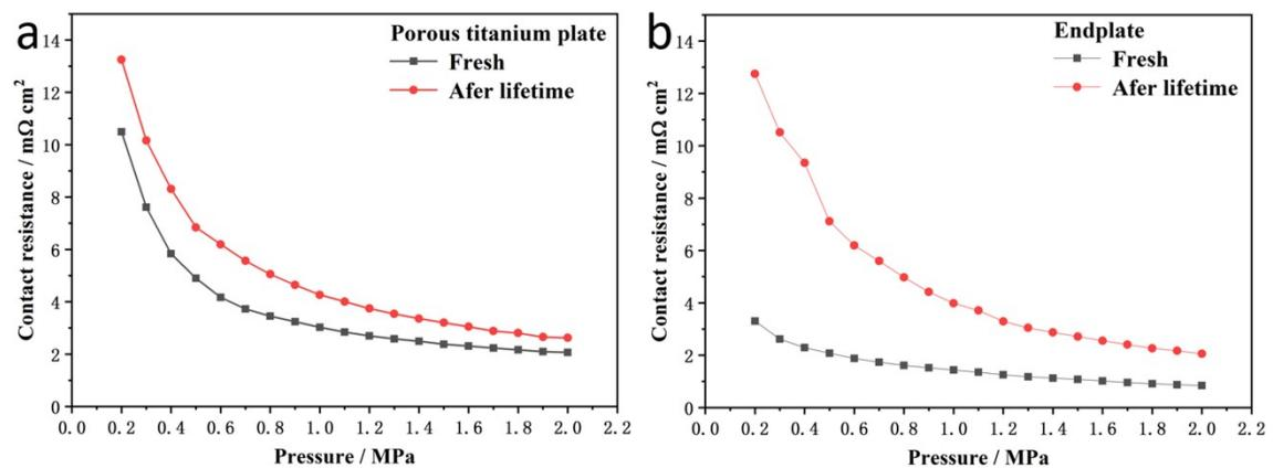
**Fig. S16** Contact resistance of (a) porous titanium plate and (b) endplate before and after the 500h lifetime.
