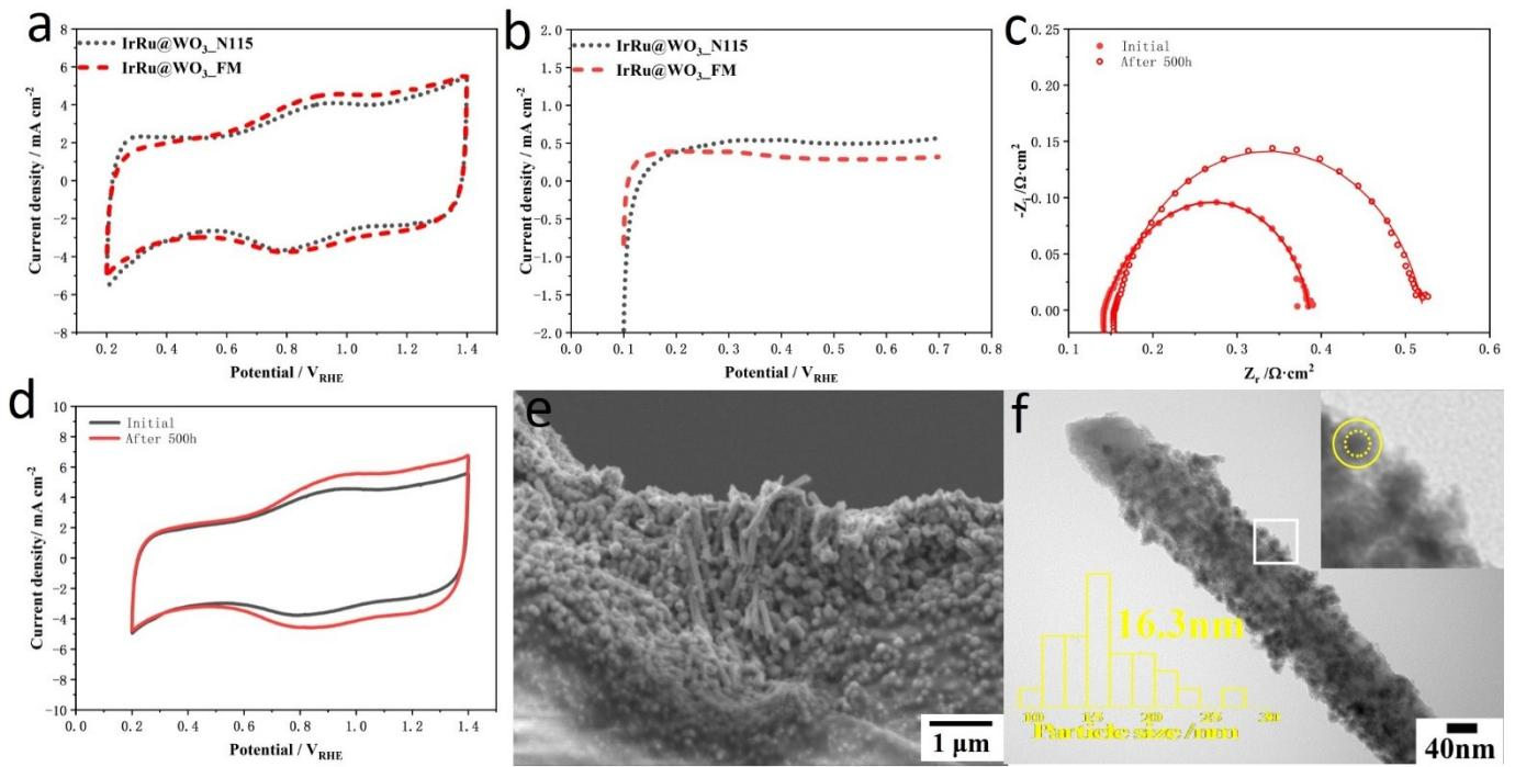
**Fig. S15.** The performance of IrRu@WO<sub>3</sub>\_N115 before and after 500 h lifetime. (a) Initial CV curve referenced to H<sub>2</sub> saturated cathode at 30 °C, (b) Initial hydrogen permeation current at 30 °C, (c) EIS curve at 1.5 V, (d) CV curves lifetime referenced to H<sub>2</sub> saturated cathode at 30 °C, (e) cross section SEM image of anode layer and (f) TEM image of anode catalyst.
