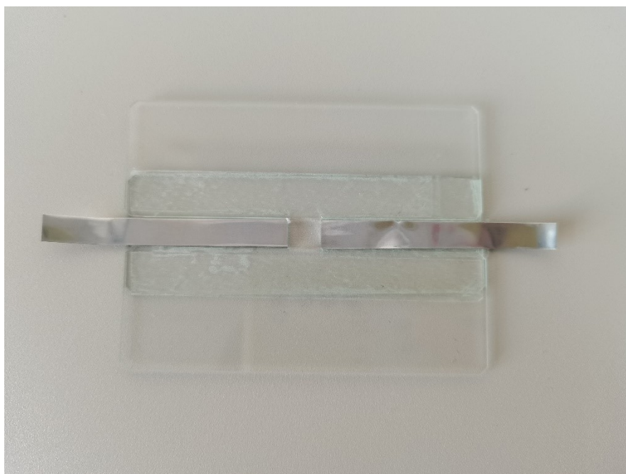
Figure S10. The photograph of Zn-Zn transparent cells for biological microscope devices.
