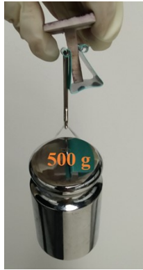
Figure S17. The T-Au/CM 0.2 sample withstanding a 500 g weight.
