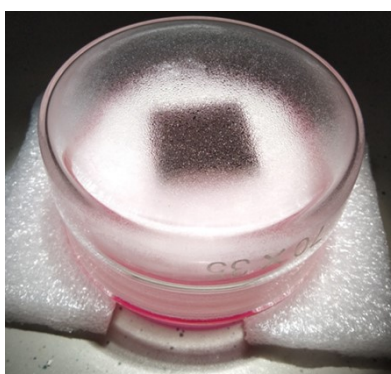
Figure S12. The condensation and collection of steam generated from T-Au/CM 0.2 device under solar irradiation.
