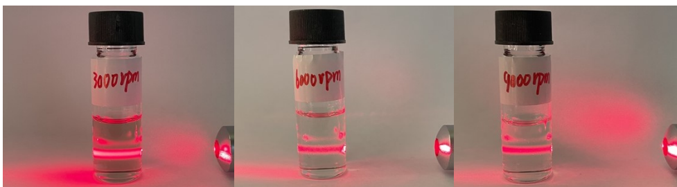
Figure S17 The Tyndall effect of the well-dispersed \text{MoS}_2 solutions with concentration of 1 mg/mL.
