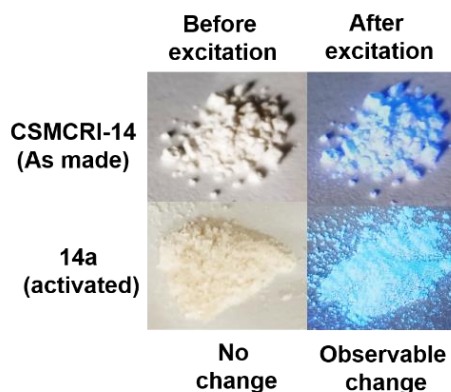
Fig. S6. (a) UV-Vis spectra of MOF constituents and activated CSMCRI-14 . (b) Comparison of emission intensity of 2-ATA, dpta , and 14a (all dispersed in water). (c) Digital photographs of CSMCRI-14 and 14a (before and after excitation).
