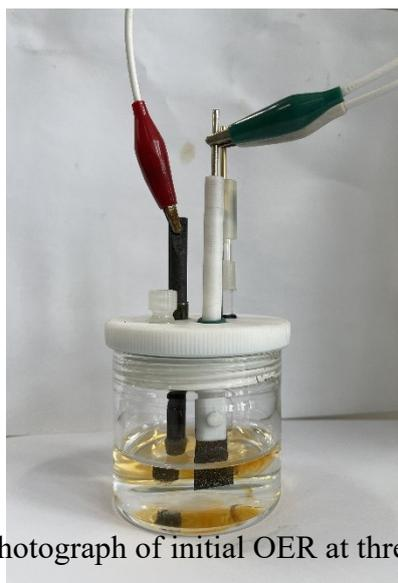
**Figure S22.** The photograph of initial OER at three electrode system.
